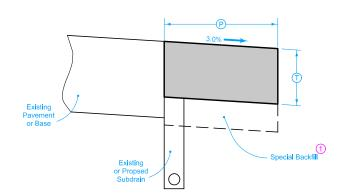
Hot Mix Asphalt Widening on Existing Pavement Without Curb
