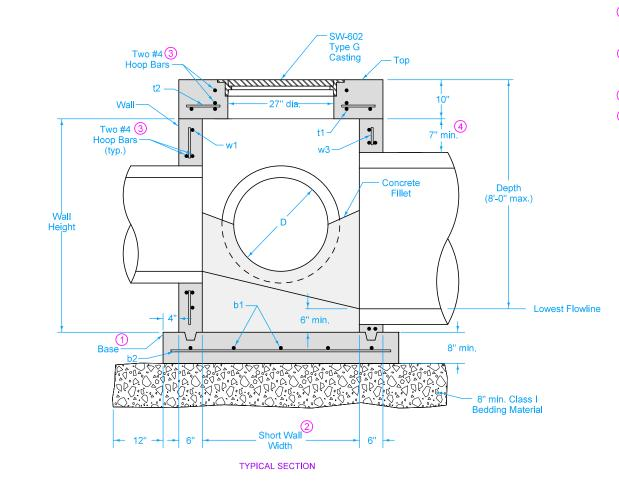
Adjacent walls may have different widths based upon pipe configuration, but structure must be rectangular.
