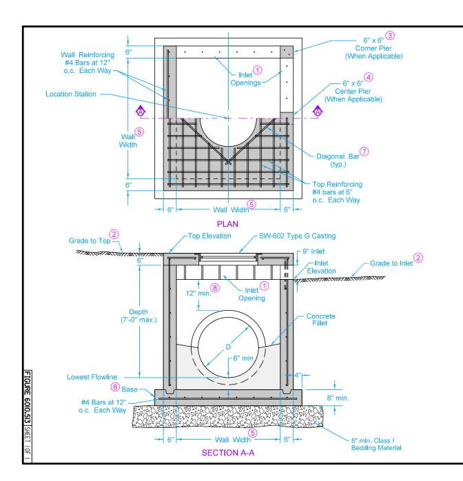
Structure may be built with openings on any or all sides. Provide openings and orientation as specified in the contract documents.
