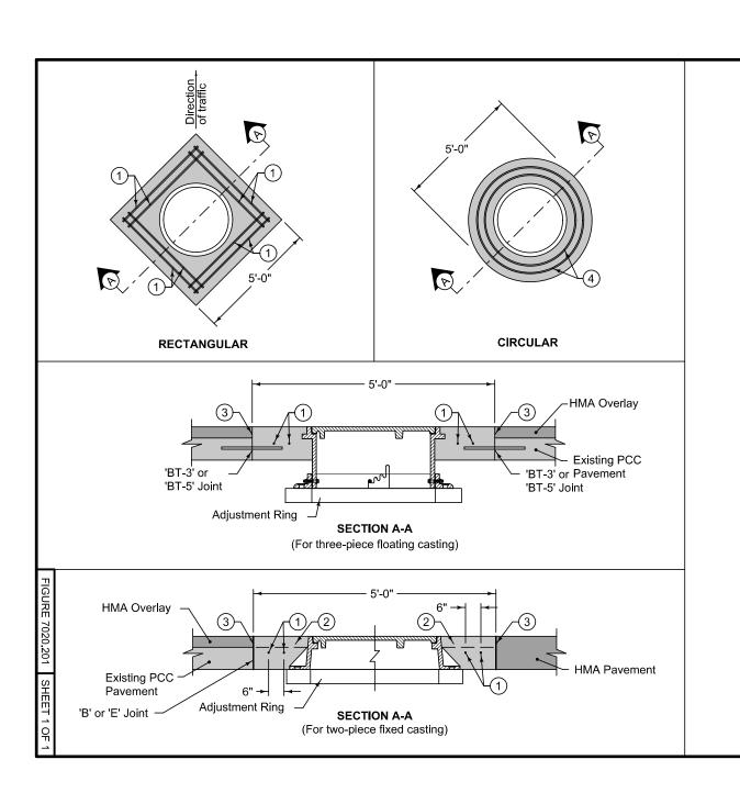
Construct boxout with Class C concrete. Minimum 2 inches clear on reinforcement. Center casting within boxout area.
