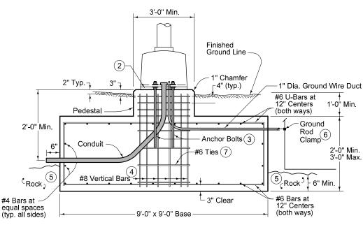
MAST ARM POLE FOUNDATION IN ROCK TYPE B FOUNDATION
