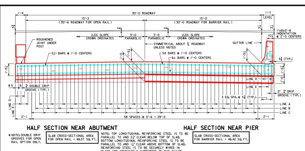
PLACE AND ADEQUATELY SUPPORTED ON BAR CHAIRS BEFORE CONCRETE IS POURED.
