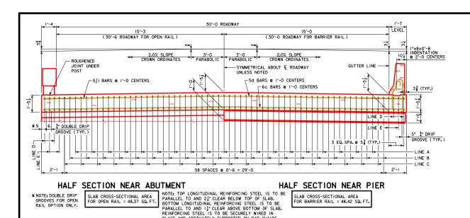
PLACE AND ADEQUATELY SUPPORTED ON BAR CHAIRS BEFORE CONCRETE IS POURED.
