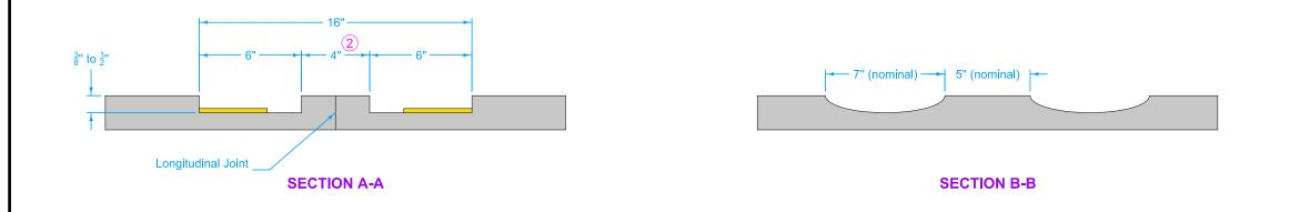
Centerline rumble strip placement is the same regardless of centerline pavement marking.
