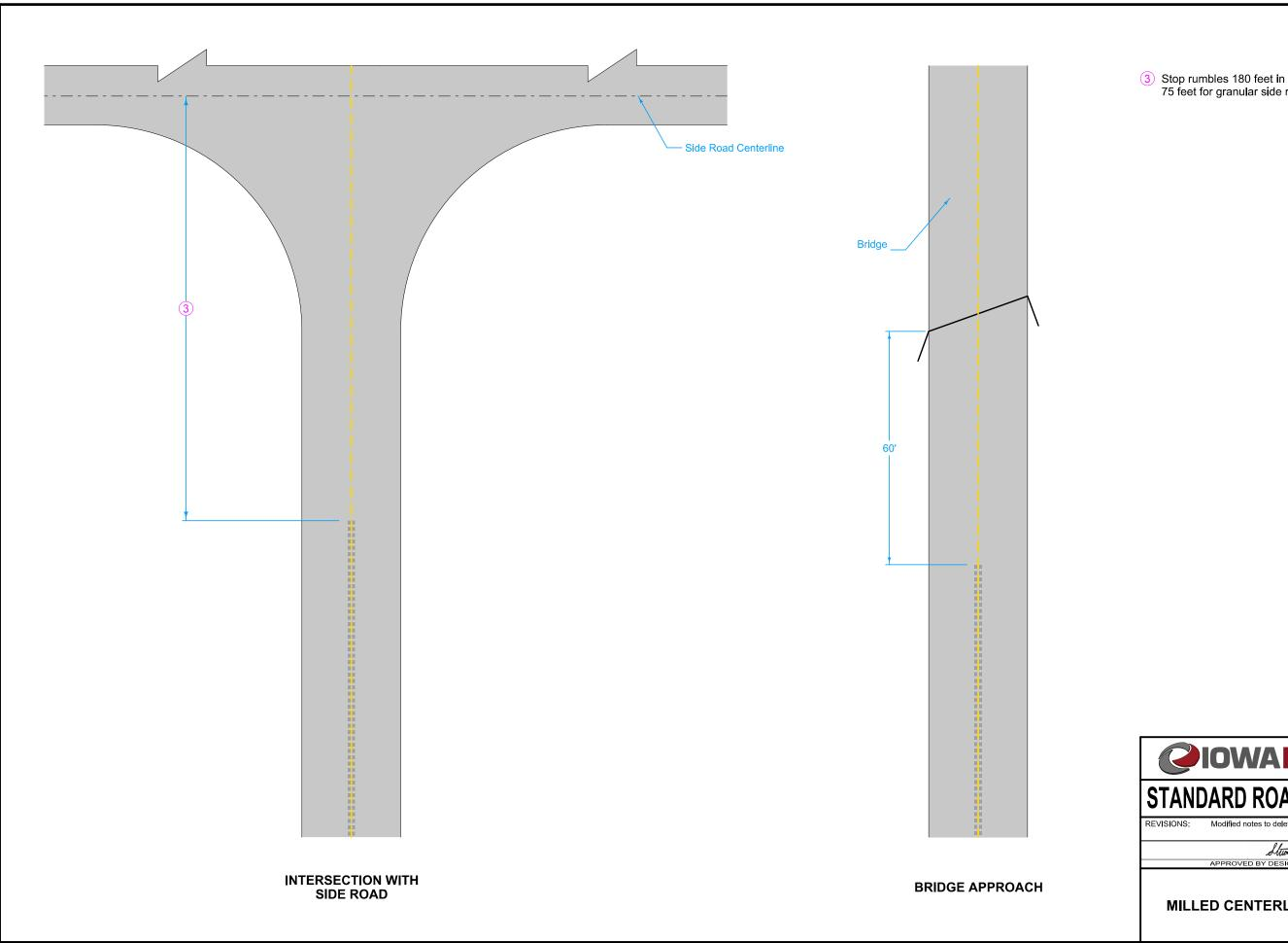
3 Stop rumbles 180 feet in advance of paved side roads or 75 feet for granular side roads.
