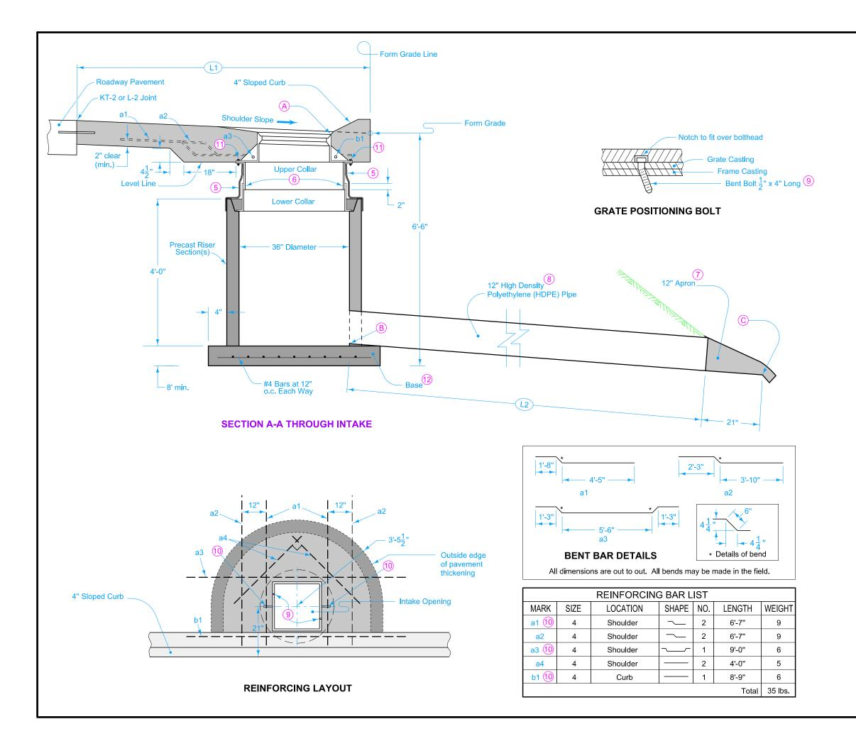
Construct precast base using 4 in. x 4 in. No. 6 steel wire mesh reinforcing or equivalent.
