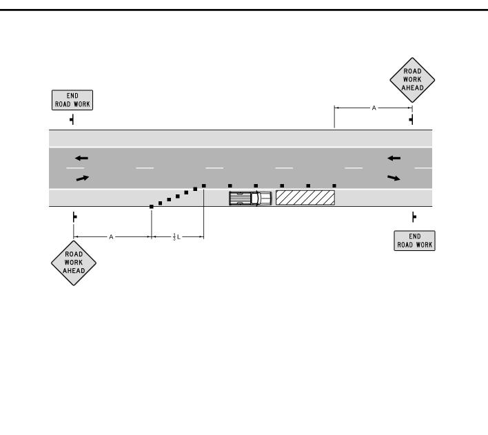
Use only on minor, low speed (≤ 40 mph) streets. Provide a lane closure for higher speed traffic conditions.
