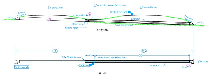
Extend on line of existing structure to Lt., Rt. or both as specified. Adapters may be required, see DR-122.
