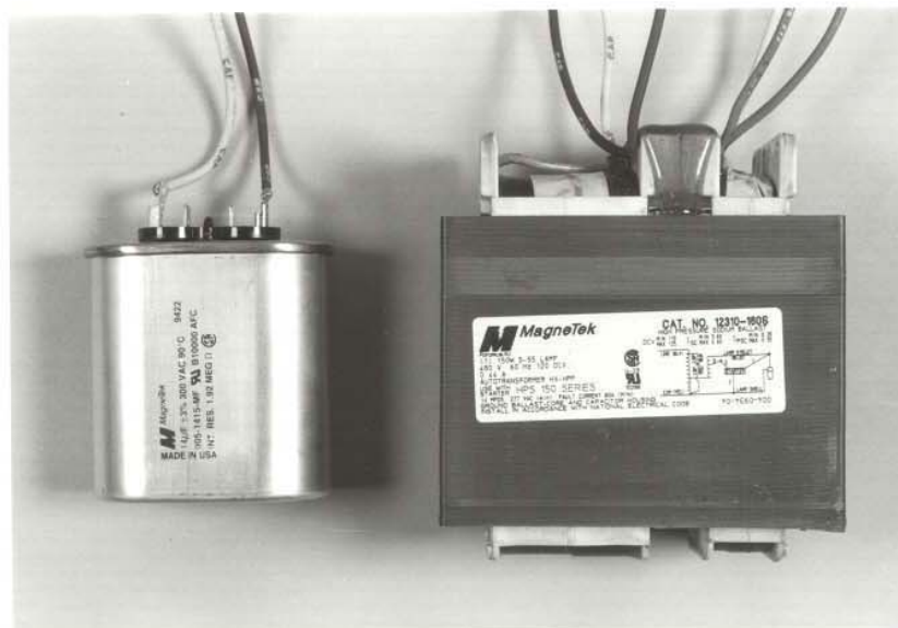
Photograph #2 Ballast unit for Mercury Vapor and Sodium Lights. Ballast unit consists of a Capacitor (left), open wound transformer (right), and starter (Photo #10).
