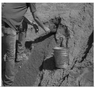
**NOTE:** Stockpile sampling of coarse *or combined* aggregate should be avoided. If it becomes absolutely necessary to obtain a sample from a *production* stockpile, consult the District Materials Engineer to help devise an adequate and proper sampling plan.
