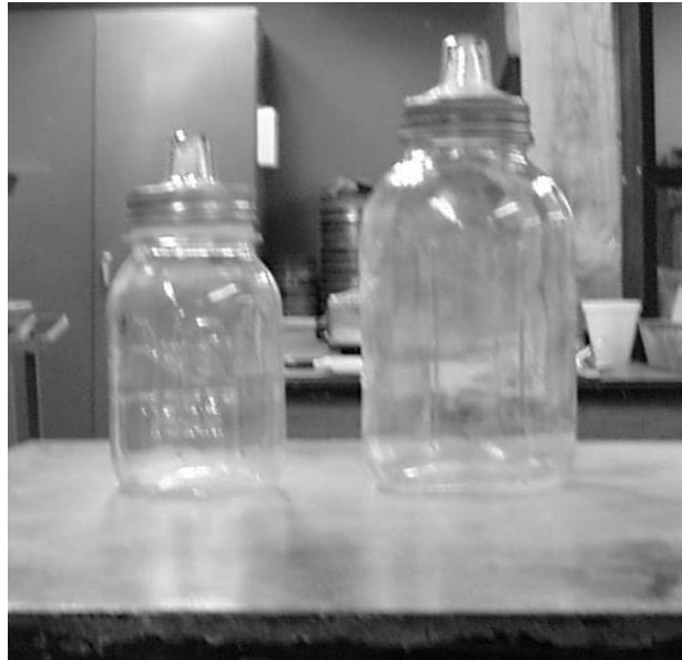
Pycnometers for Coarse and Fine Aggregates
