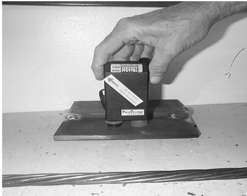
Figure 1. Operation of Film Thickness Gauge
