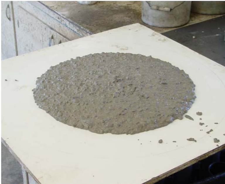
Figure 2. Slump Flow Visual Stability Index of 0 – This is a high quality SCC with a Visual Stability Index of 0. There is no indication of segregation or separation. Aggregate distribution is good and particles are carried to the outer edge of the slump flow.
