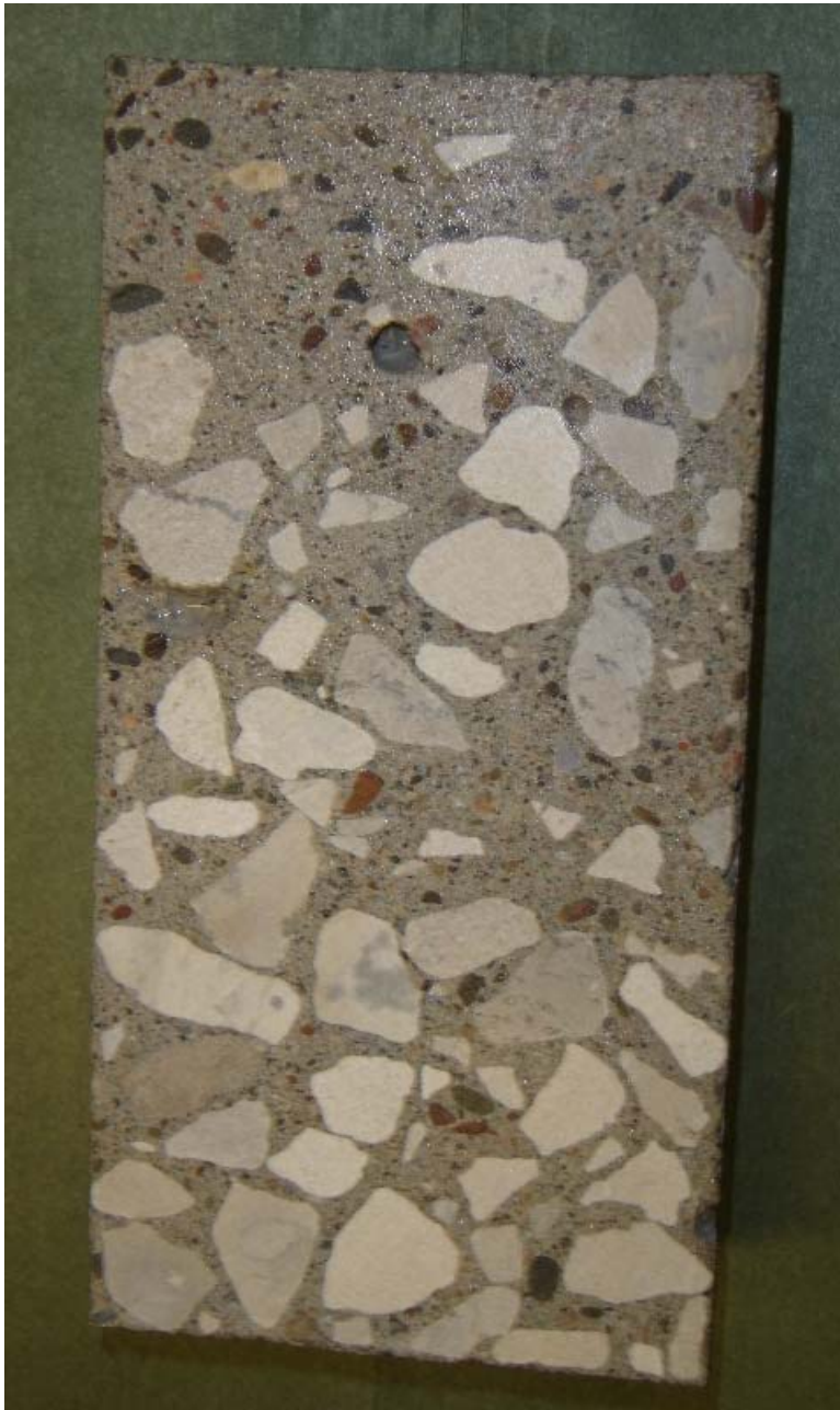
Figure 2. Hardened Visual Stability Index (HVSI) = 3. Note mortar layer greater than one inch at surface and coarse aggregate distributed in lower half.
