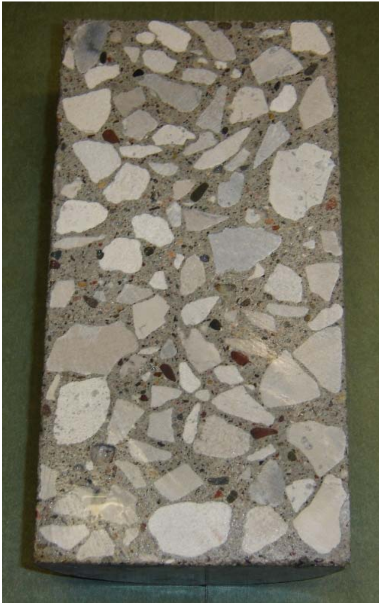
Figure 1. Hardened Visual Stability Index (HVSI) = 0. No mortar layer coarse aggregate well distributed.
