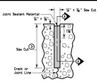
**DETAIL "A"**(Sawcut formed by conventional concrete saving equipment)
