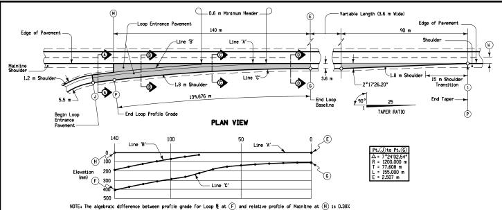
Loop exit pavement shall be the same thickness as mainline pavement.
