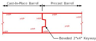
Joint Detail at Cast-In-Place Barrel Connection
