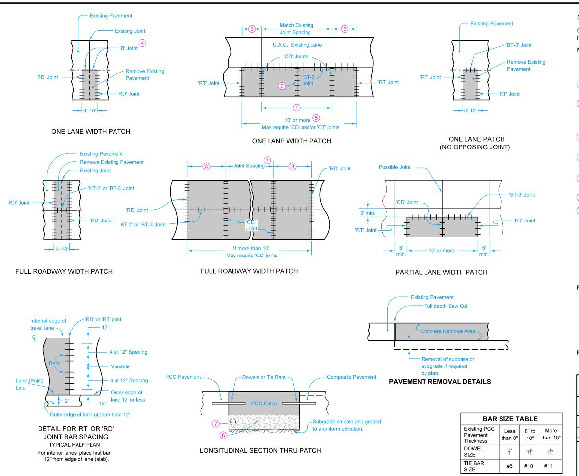
See PV-101 for joint and bar placement details.
