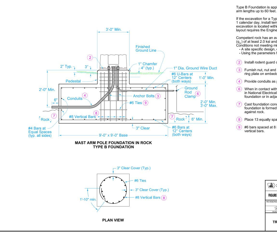
FIGURE <u>8010.102</u> SHEET <u>2</u> OF <u>4</u> Type B Foundation is applicable for traffic signal poles with mast
