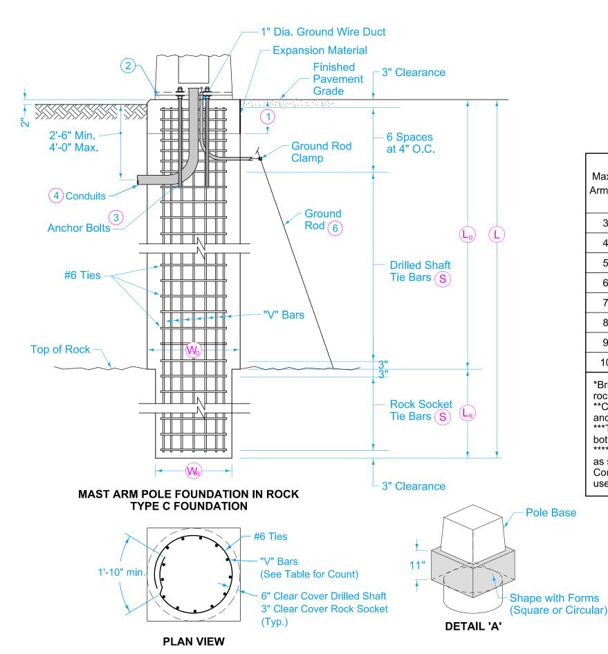
(1)(2)Install rodent guard or non-shrink grout with weep hole. (3) Furnish nut, nut and plate, or nut and anchor bolt assembly ring plate on embedded end. (4) Provide conduits as per plans. (6) When in contact with rock, place ground rods as specified in National Electrical Code, current edition, adjacent to foundation or in adjacent handhole.
