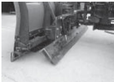
Slush blades made of one-and-one-half-inch rubber will be added behind the normal carbide snow plow blade and tested for its
