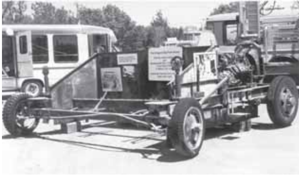
The final Iowa State Highway Commission slipform paver could pave one lane of traffic in a single pass. Circa 1949
