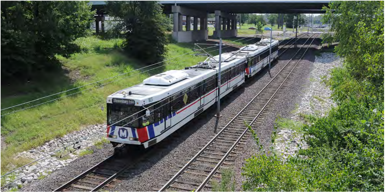
Figure 3.14: Typical LRT Operations in Dedicated Right-of-Way
