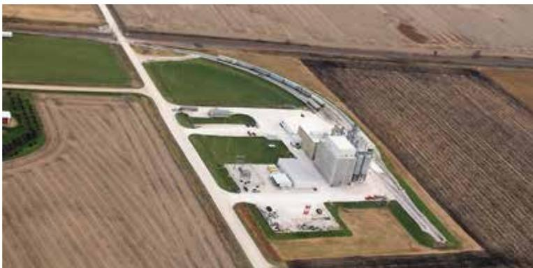
Prior to this project, Iowa Corn Processors (ICP) was served by a single track that was approximately 1,800 feet in length. That set-up required the serving railroad to make multiple entries and exits to the property to deliver empty cars and take away loaded cars. This was inefficient for the railroad because it tied up their main-line tracks causing congestion along the system.
