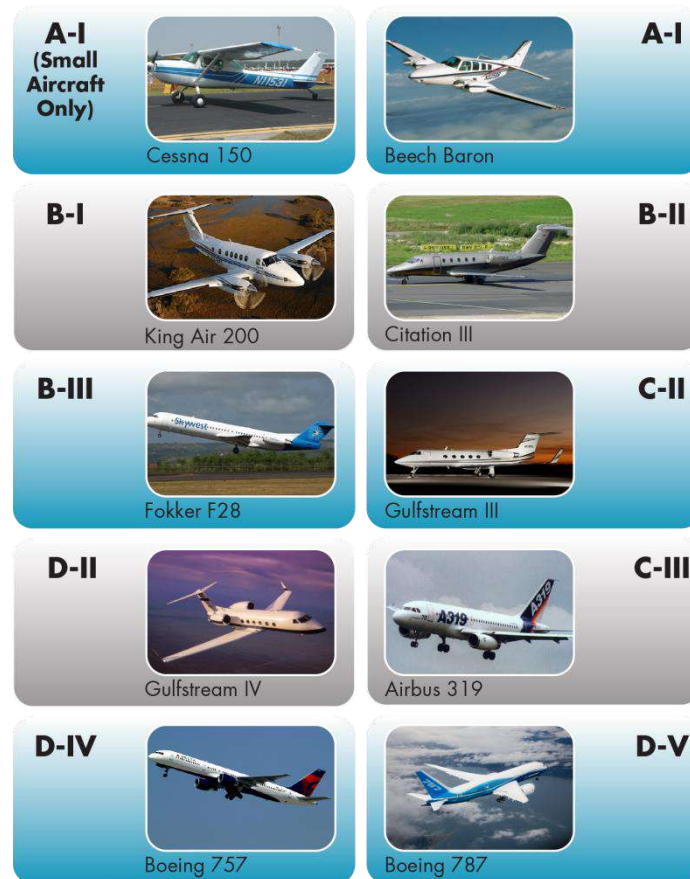
Figure 2-6: Runway Design Code Aircraft Types AIRPORT REFERENCE CODE (ARC)
