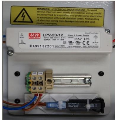
Figure 14: AC power supply terminal block
