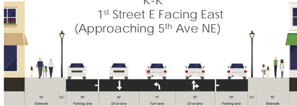
K-K 1 st Street EB One-Way Lane Reconfiguration
