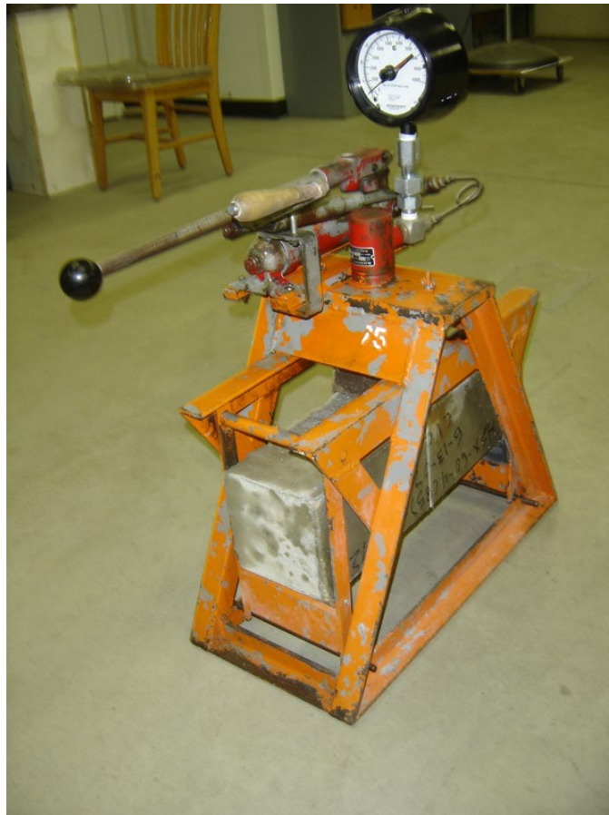
Figure 2. Six Inch Concrete Specimen in Hydraulic Testing Machine
