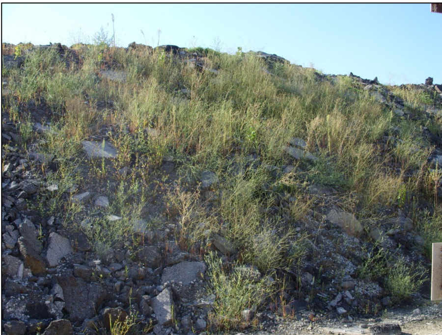
Figure 2. Recycled stockpile contaminated with organic material.
