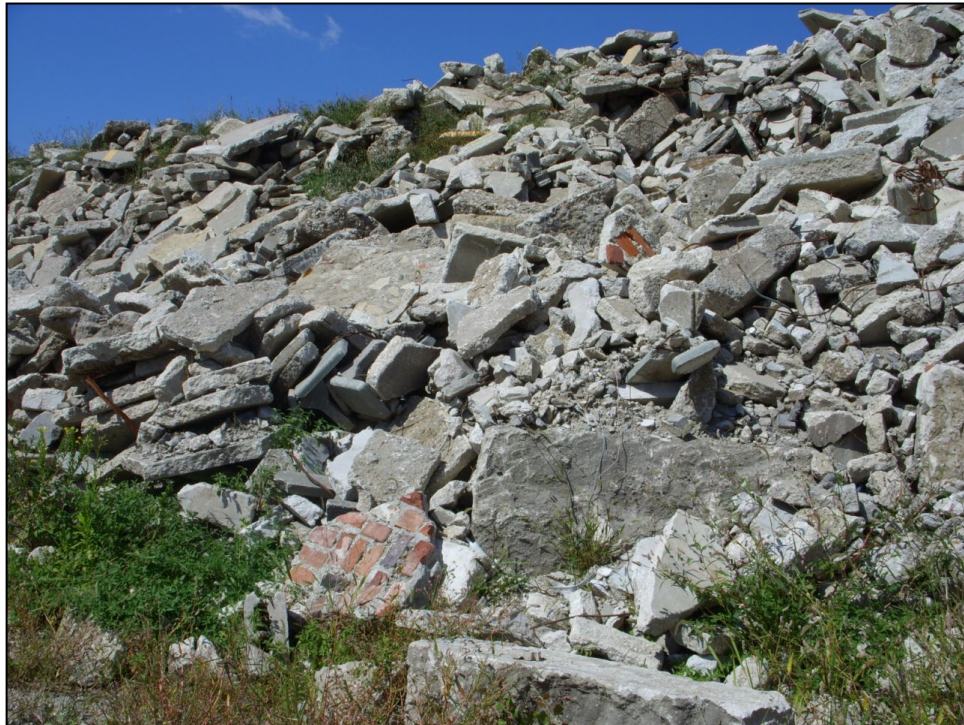
Figure 4. Recycled stockpile contaminated with non-pavement material.
