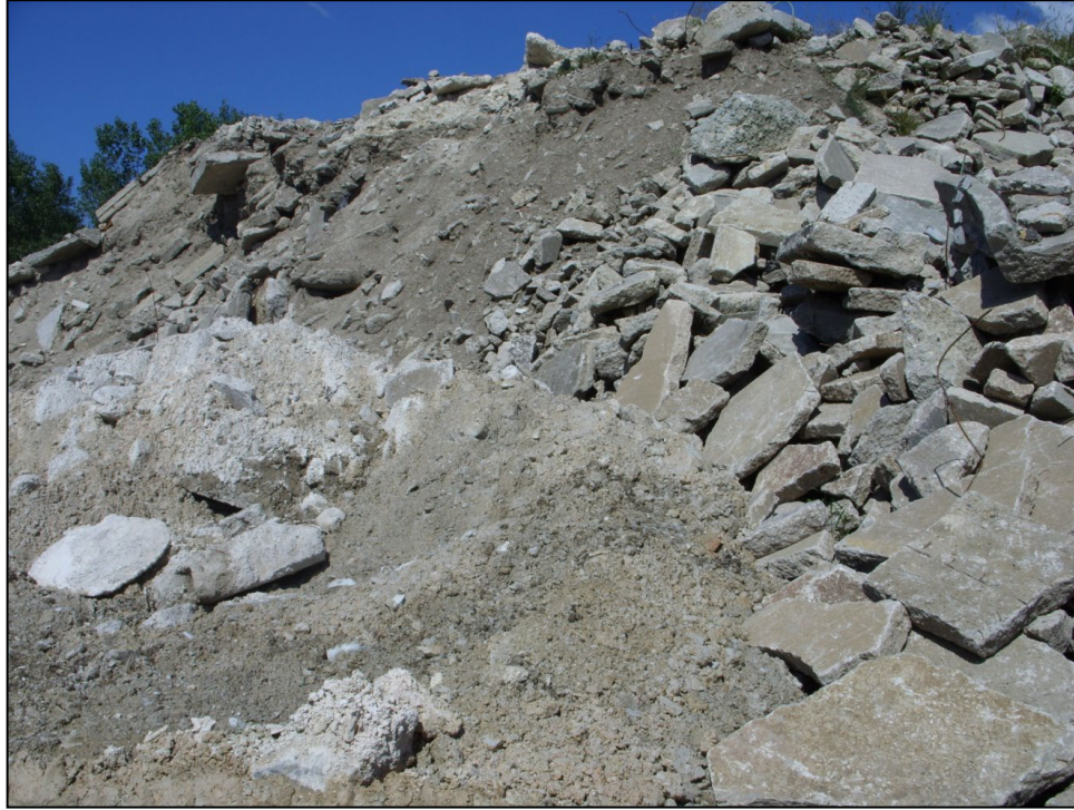
Figure 3. Recycled stockpile with excessive fines.
