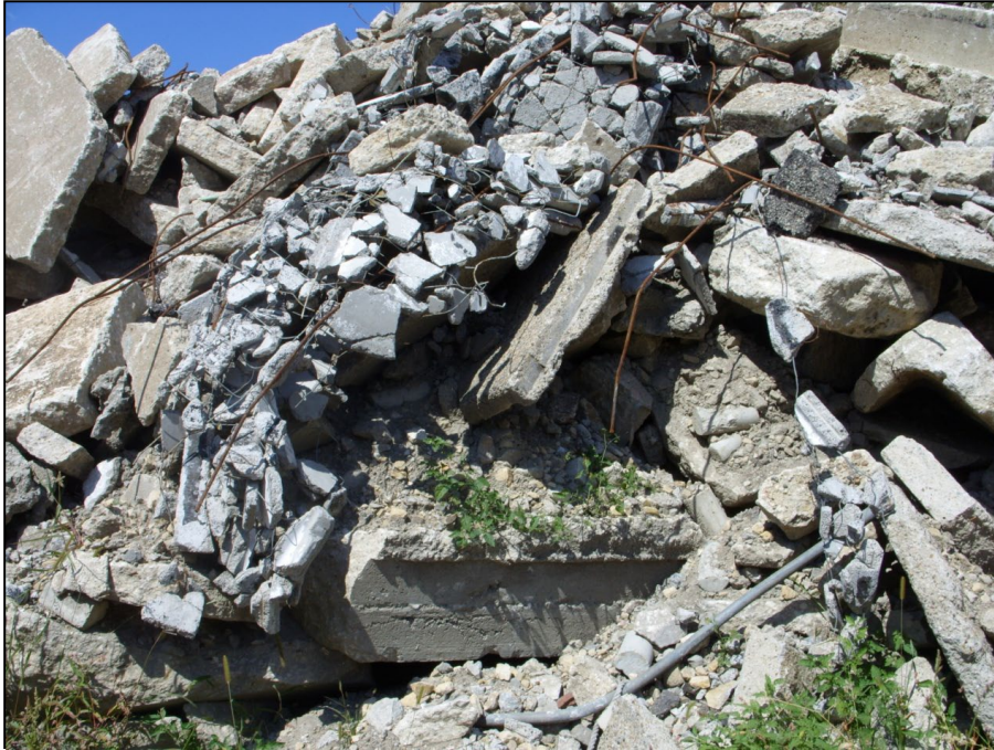
Figure 1. Recycled stockpile contaminated with steel
