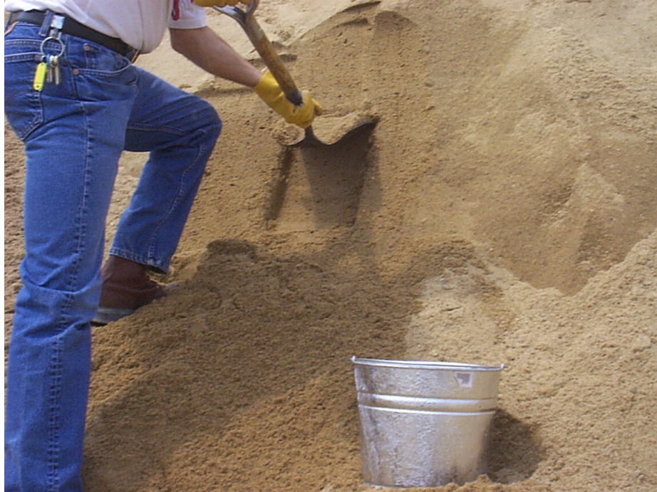
Stockpile sampling using a shovel.
