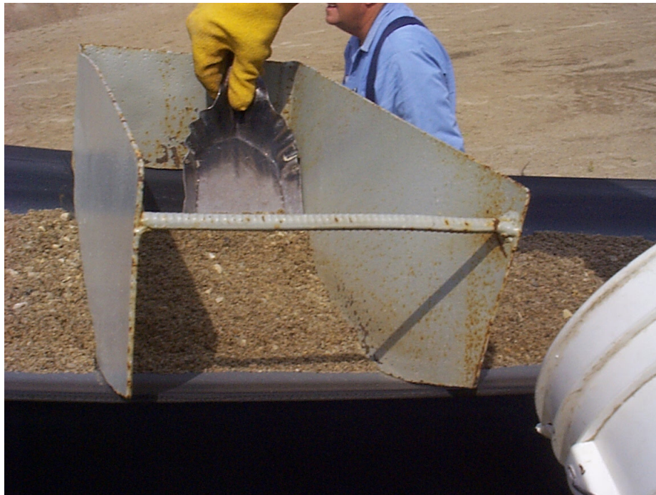
Sampling from a conveyor belt using a template
