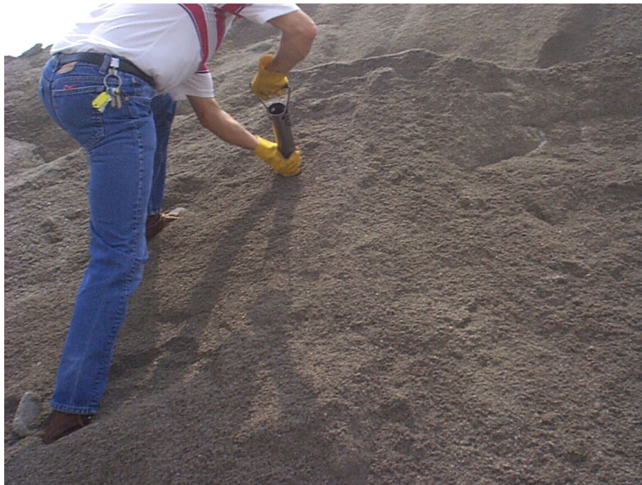
Stockpile sampling using a sand probe.
