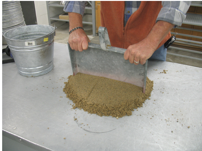
Quartering using straight edge.
