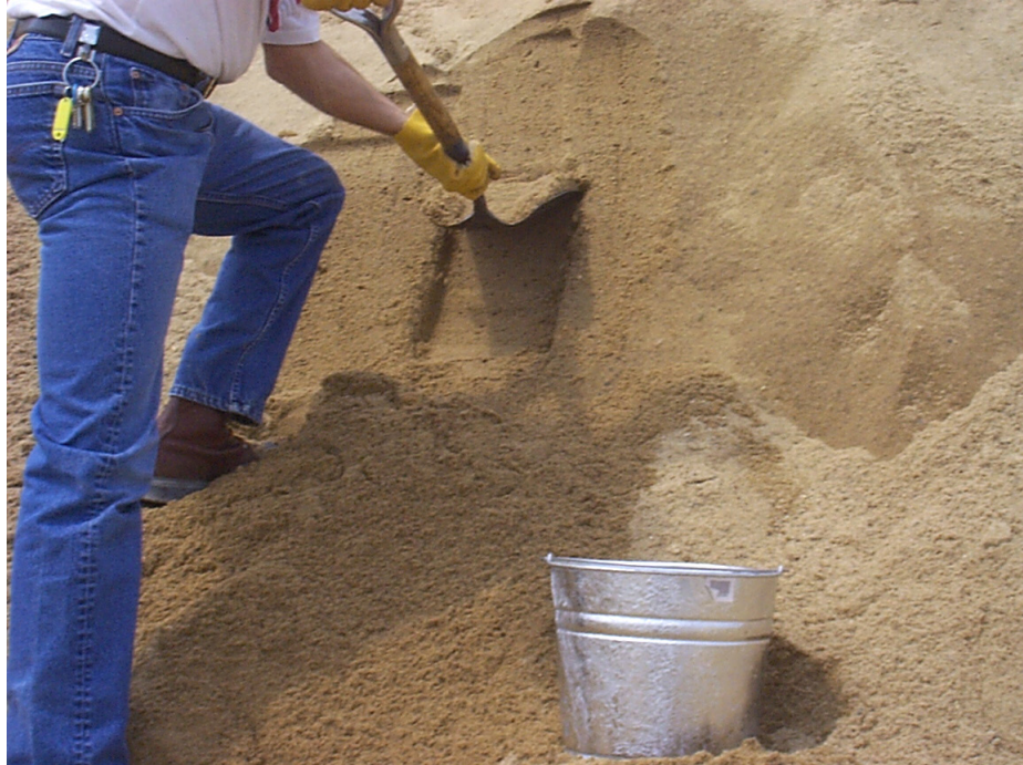
Stockpile sampling using a shovel.
