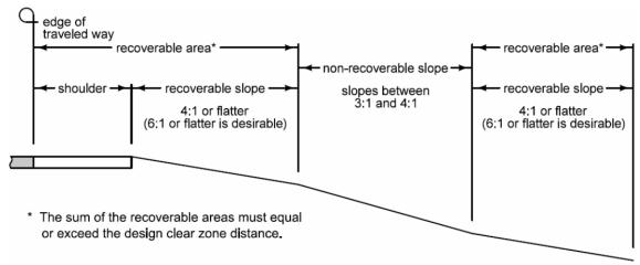
Figure 5: Example of a non-recoverable foreslope design.
