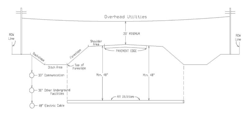
On rural-type roadways, a permanent, aboveground obstruction is to be situated as near to the right-of-way line as practical in an area beyond the clear zone or the road foreslope, whichever area locates the obstruction a greater distance from the edge of the traveled way, right-of-way width permitting.
