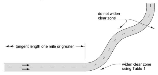
Figure 7: Clear zone adjustment at horizontal curves.
