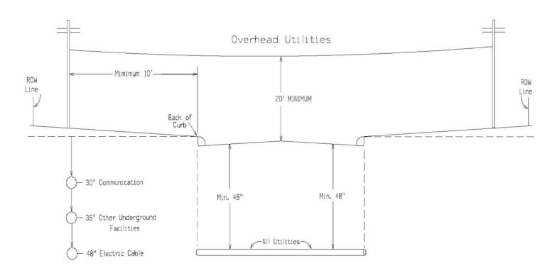
On urban-type roadways, the face of a permanent, aboveground obstruction is to be situated no closer than 10 feet from the back of the curb. In areas with parking or auxiliary lanes, an aboveground obstruction is to be situated no closer than two feet behind the back of the curb or a minimum of 10 feet from the edge of the traveled way, whichever location is farther from the traveled way.
