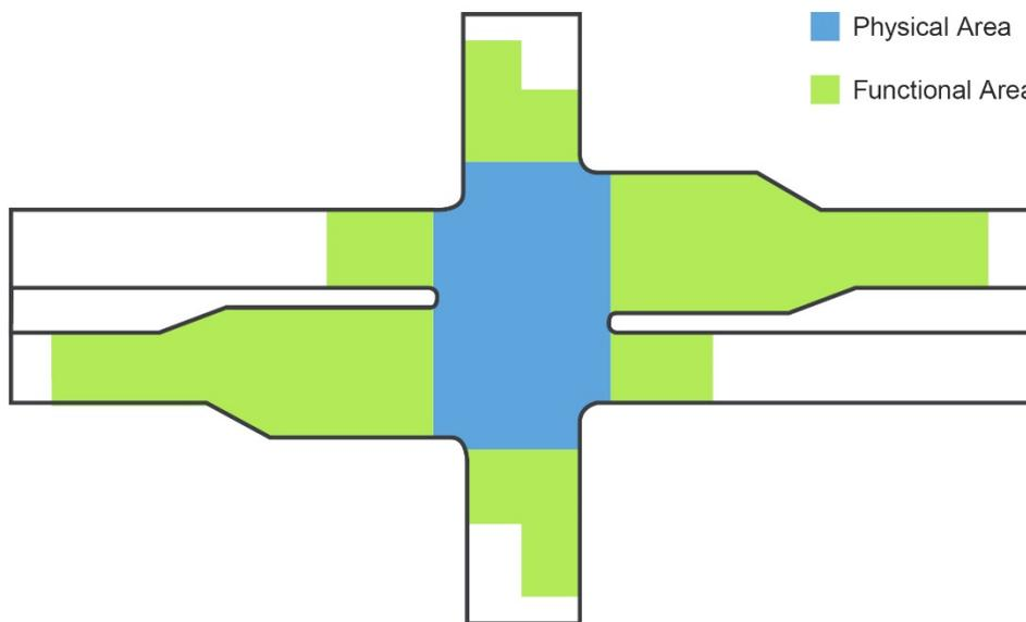
**Figure 2.2 – Physical and Functional Areas of an Intersection**
