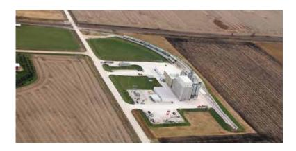
Prior to this project, lowa Corn Processors (ICP) was served by a single track that was approximately 1,800 feet in length. That set-up required the serving railroad to make multiple entries and exits to the property to deliver empty cars and take away loaded cars. This was inefficient for the railroad because it tied up their main-line tracks causing congestion along the system.
