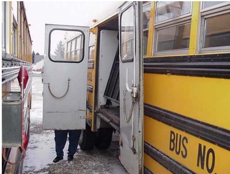
Figure 10. External view of wheelchair door
