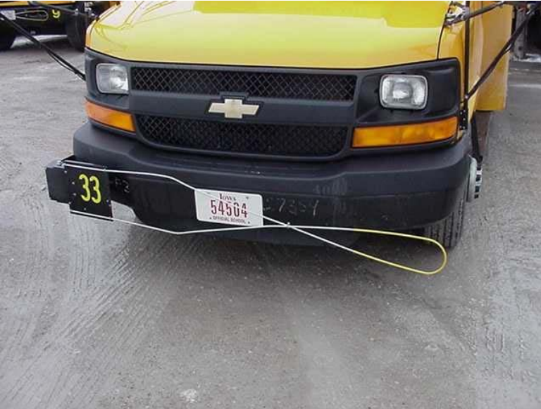
Figure 13. Crossing control arm (courtesy of Ankeny School District)
