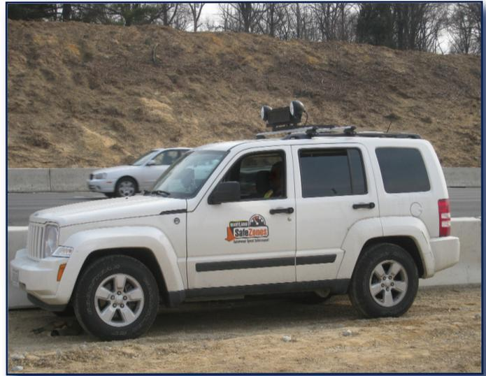
Examples of Semi-Automated Work Zone Speed Enforcement Vehicles
