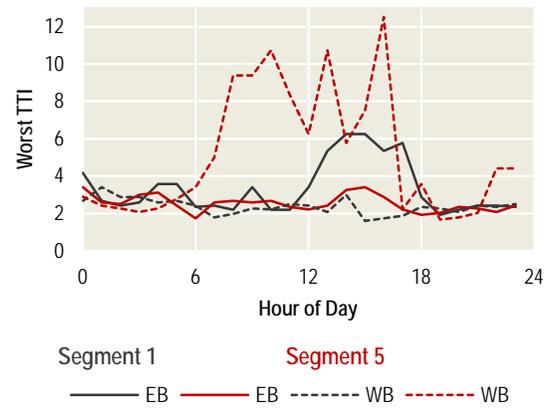
**Figure E.10. Existing (Field-Measured) Cumulative Time Travel Index Curves**
