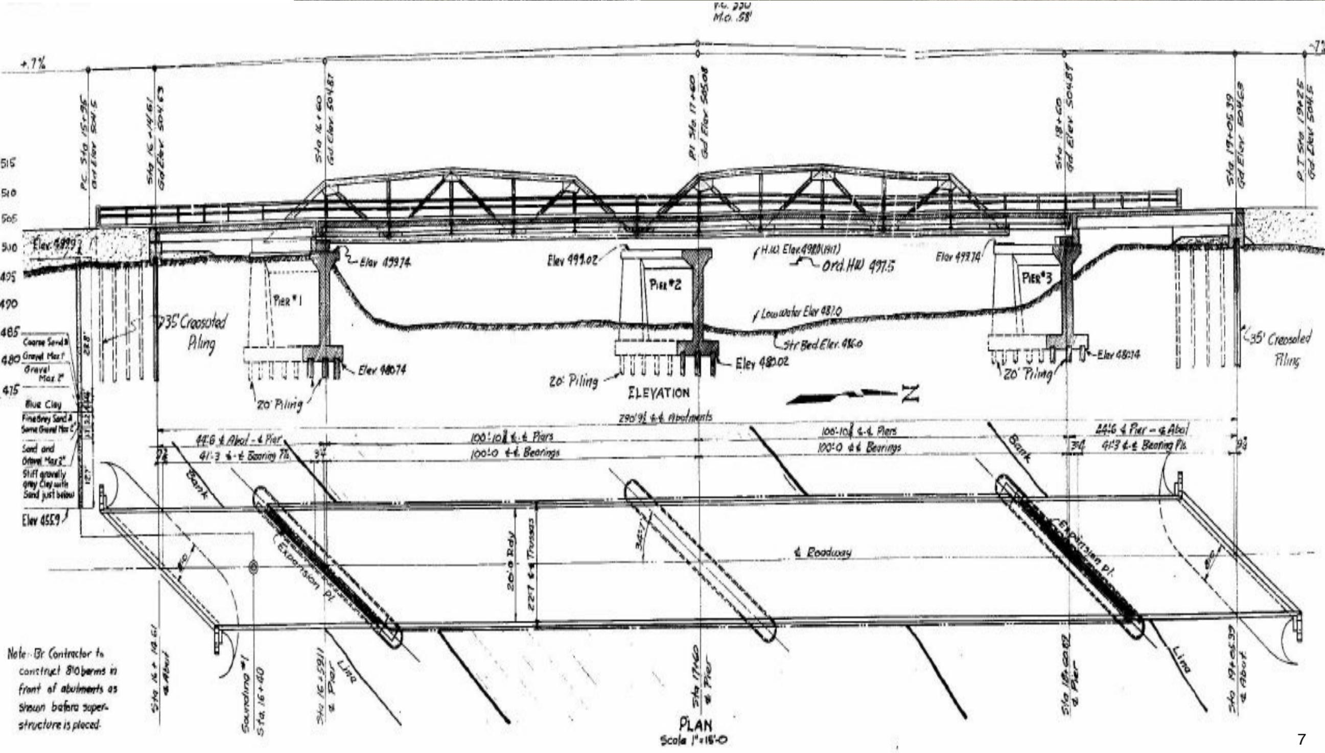
Right: Iowa State Highway Commission Standard Design Plans for the Nishnabotna River Bridge, shown in plan and elevation.
