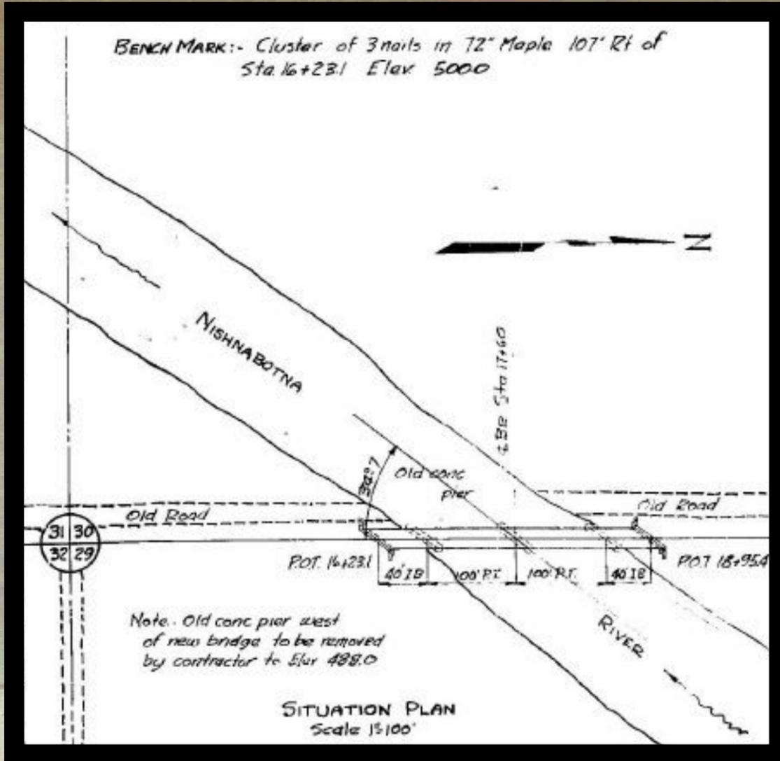
Above: Situation plan from the Iowa Highway Commission Standard Design Plans for the Nishnabotna River Bridge. These plans depict the adjustments engineers made to accommodate the river channel and flow patterns.
