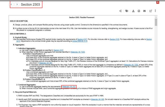
4. Place stockpiles of RAP as directed in <u>Materials 1M. 505</u>. Do not use RAP stockpiles containing concrete chunks, grass, dirt, wood, metal, coal tar, or other foreign or environmentally restricted materials. RAP stockpiles may include PCC (not to exceed 10% of the stockpile) from patches or composite pavement that was milled as part of the asphalt pavement.
