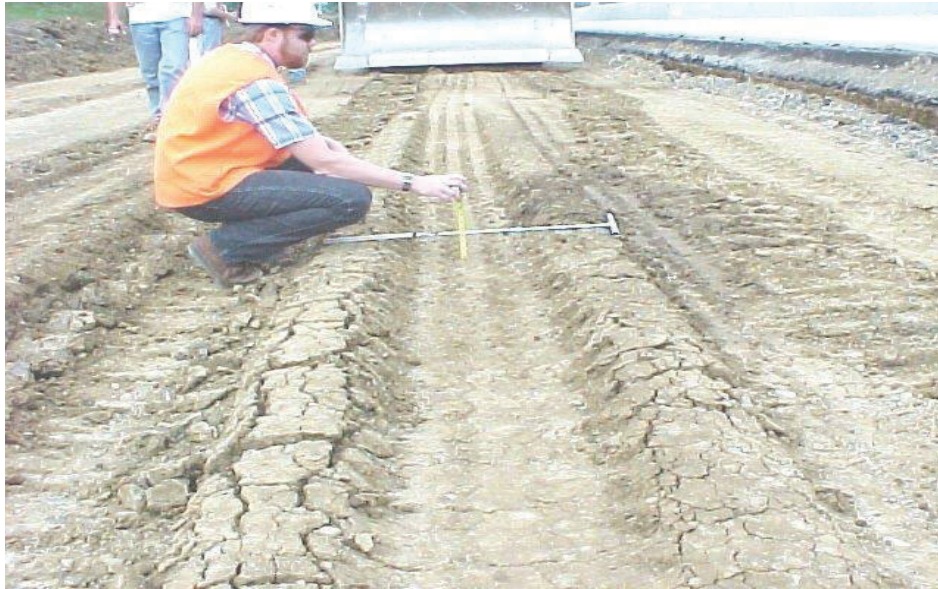
Figure 12-1: Inspector measuring ruts following the proof-roll test.
