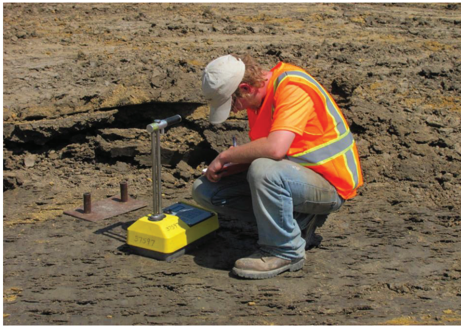
Figure 6-9: Nuclear gauge test used to determine in-place density of a compacted lift.
