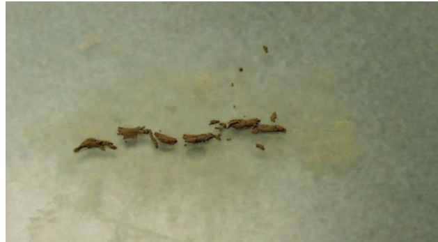
Figure 2-6: Test to determine plastic limit of soil.
