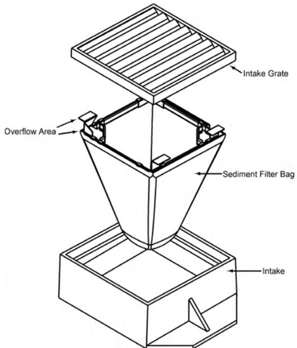
**This type of inlet protection uses a sediment filter bag**
