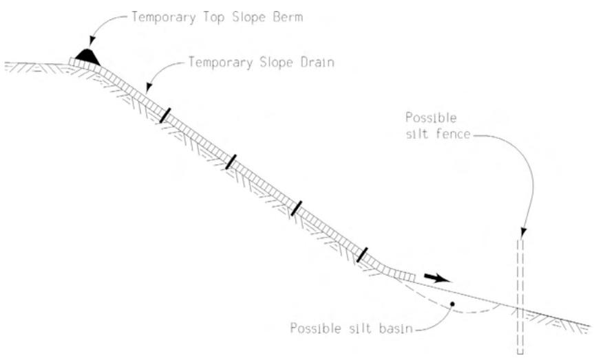
**Plan and profile of a temporary slope drain.**
