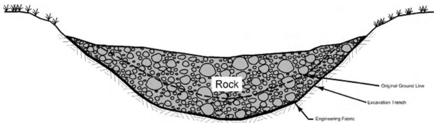
**Rock Check Dam detail for temporary applications.**
