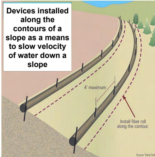
EC-204 shows installation requirements, including proper staking and stapling. **Please be aware** that photos included in this guide show previous staking requirements with the stake going through the device.
