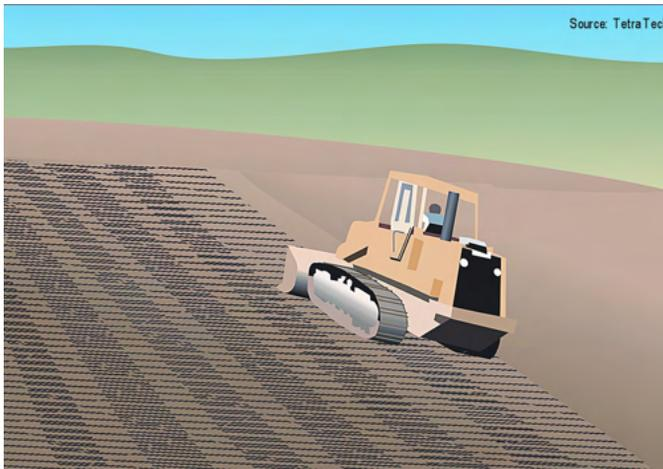
**Dozer tracking is created by equipment moving up and down a slope rather than along the contour.**
