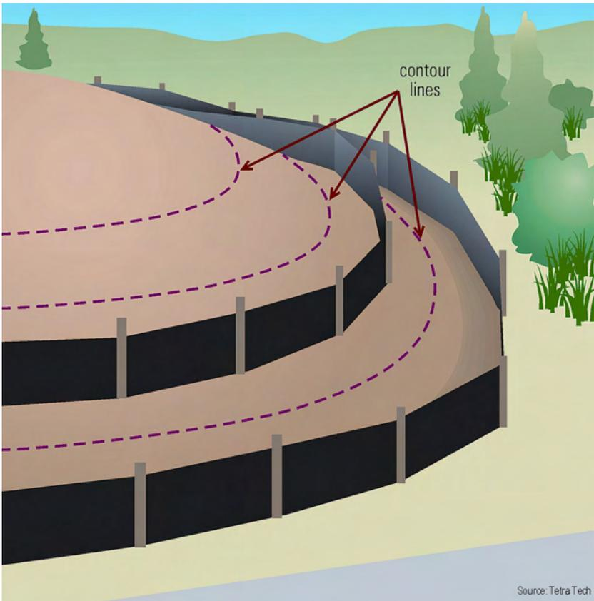
**This illustration shows multiple rows of silt fence installed along the contour lines.**
