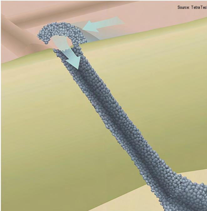
**A letdown flume is installed to direct water from an intercepting ditch down a slope without causing erosion.**
