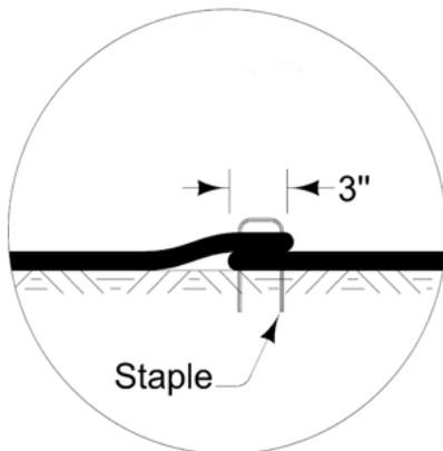
**When a new section is added, it should be placed 3 inches over the previous section of fabric and stapled in place.**
