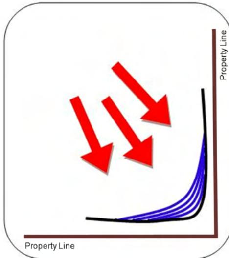
**This is an incorrect layout of silt fence installed as perimeter control along a property line. Run-off will concentrate in the lower right corner and overwhelm the silt fence, and a blow-out will occur.**
