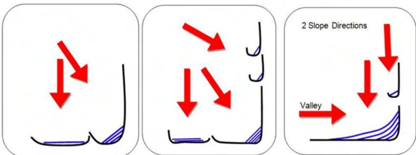
**These are examples of correct silt fence placement where a single section of silt fence is broken up into multiple sections with J-hooks. Multiple sections provide multiple storage areas for water to accumulate, thus reducing the chance of a blow-out.**
