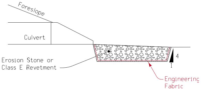
**Detail of splash basin at a culvert.**
