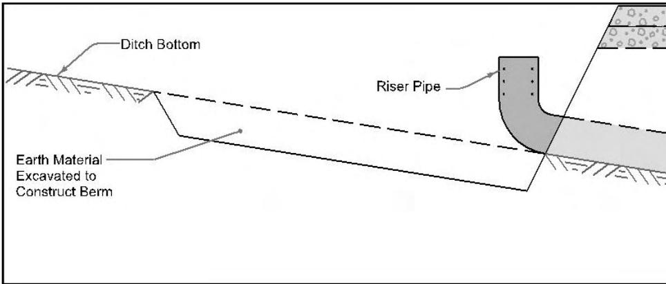
**Profile of a temporary sediment control basin.**
