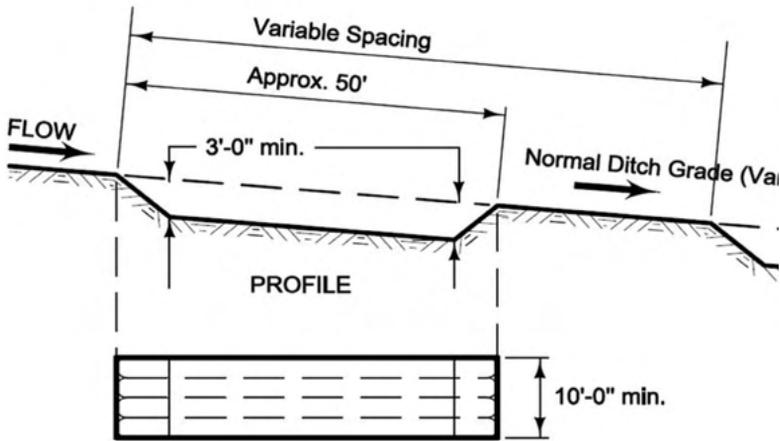
**Detail of a silt basin - Notice that the length is longer than the width. This is to allow more time for sediment to settle out prior to flows being discharged from the basin.**
