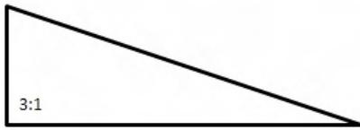
$$\begin{aligned} V/H &= \% \text{ Slope} \\ 1/6 &= .16 \text{ (16\%)} \\ 1/3 &= .33 \text{ (33\%)} \end{aligned}$$
