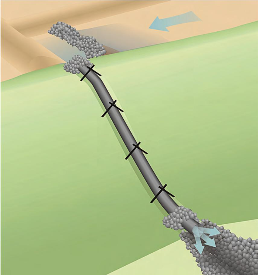
This illustration shows a temporary slope drain. Though not commonly used in Iowa, other states have used this type of control to convey water through a pipe over a disturbed slope.
