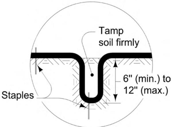
**Check slots should be used in ditches with slopes of more than 4%.**
