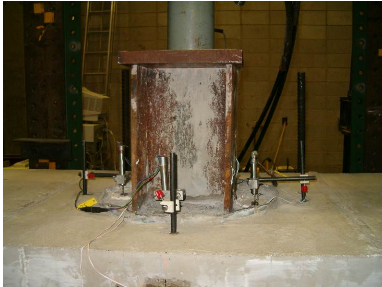
Figure 3 – Laboratory Load Testing Pile to Precast Concrete Abutment Connection
