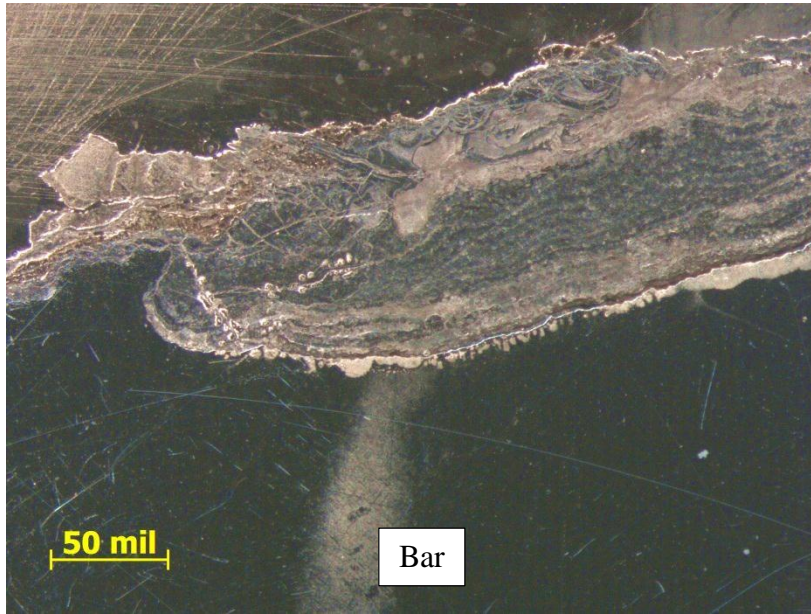
Figure 35. Cross-section of Sample 10, showing the corroded bar and pitting corrosion.
