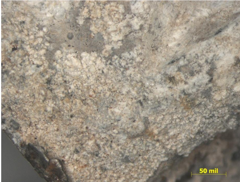
Figure 19. Micrograph of the bottom surface of Sample 10, showing a white deposit.
