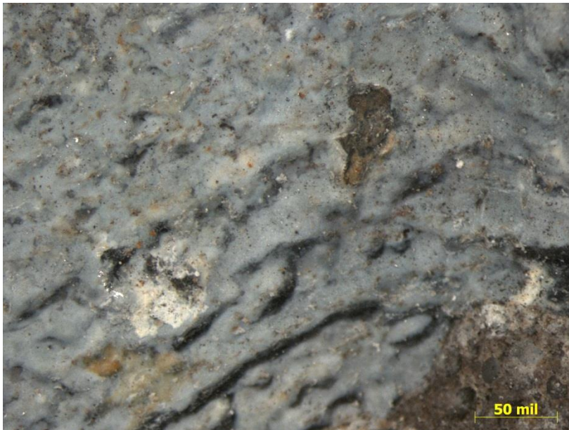
Figure 20. Micrograph of the blue-gray deposit on the side of Sample 10.
