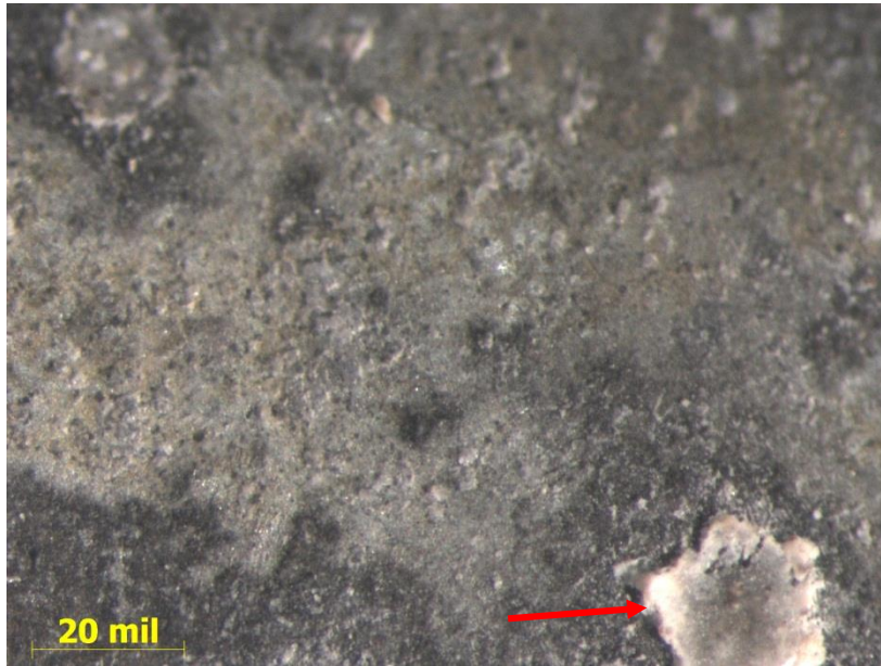
Figure 3. Micrograph of the bottom side of Sample 8. Note the dark to light coloration, with some white deposit indicated with an arrow.
