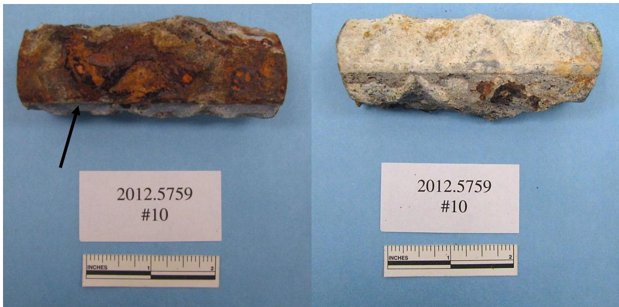
Figure 16. Sample 10. Top side (left) and bottom side (right). The stripe of blue-gray deposit is indicated with an arrow.
