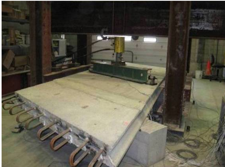
Figure 2.26. Laboratory setup for Panel 3 ultimate load test
