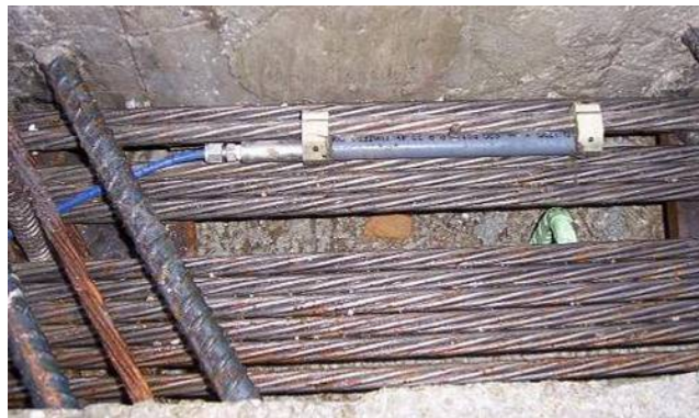
Figure 84. PT strand vibrating wire gage
