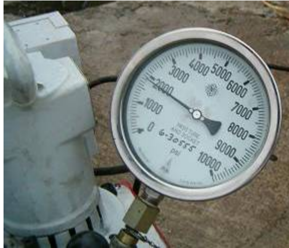
Figure 90. Hydraulic mono-jack gage
