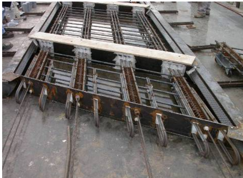
b) Double hooks and prestressing strands
