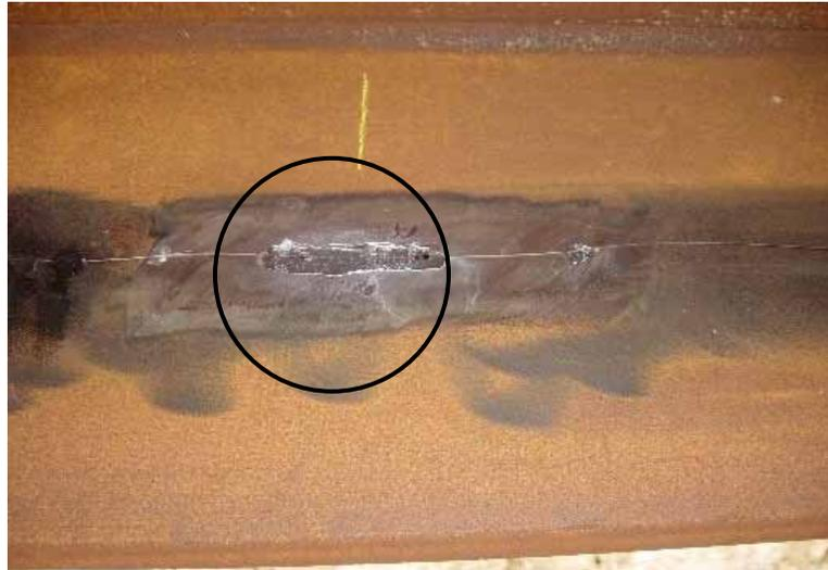
**Figure 4.8. Single bare FBG sensor after installation**
