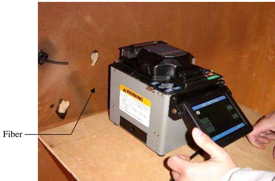
**Figure 4.11. Fusion splicing of two fibers**
