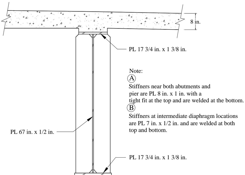
**Figure 3.5. Cross section of “Center Region” girders**
