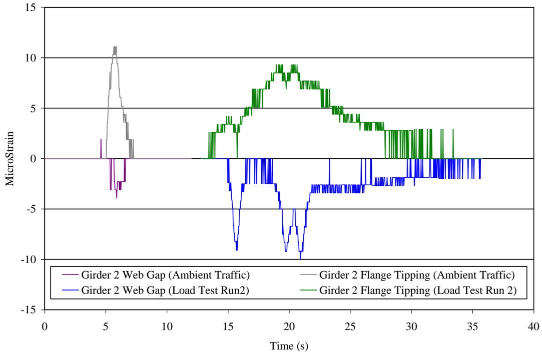
**Figure 5.18. Girder 2 web gap comparison for Ambient Traffic Event 1 and run 2**
