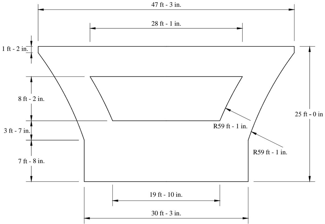
**Figure 3.12. Elevation view of the center pier**
