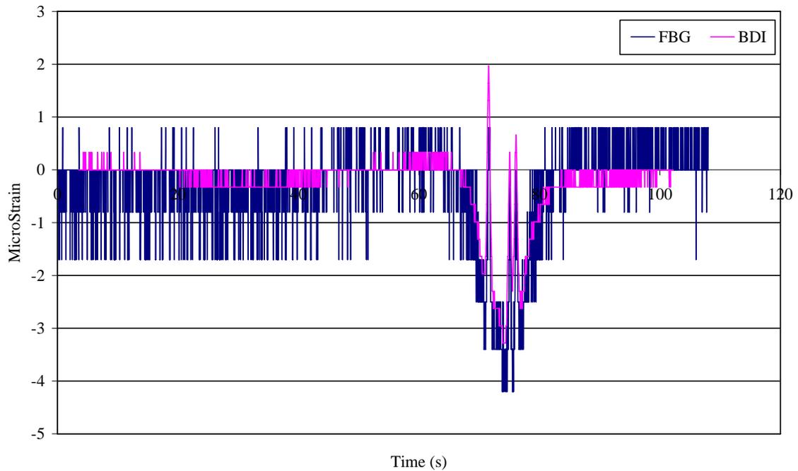
**Figure 5.7. FBG and BDI strain comparison from the top flange of girder 4 at the south midspan, run 3 of the controlled load test**
