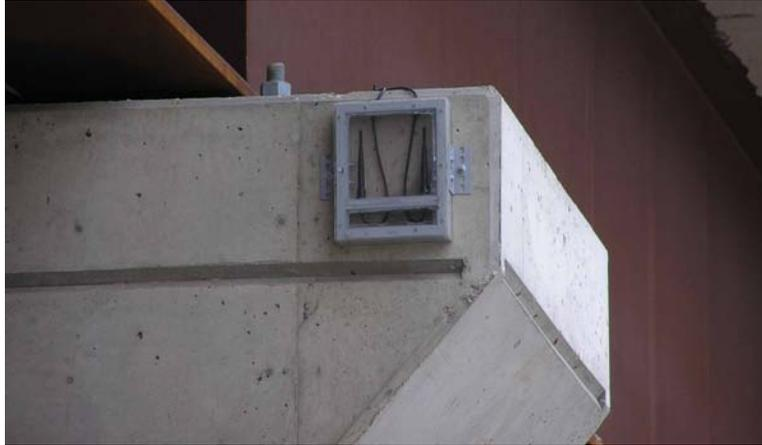
**Figure 4.18. Data acquisition sub-system WAP antennas placed at the edge of bridge pier**
