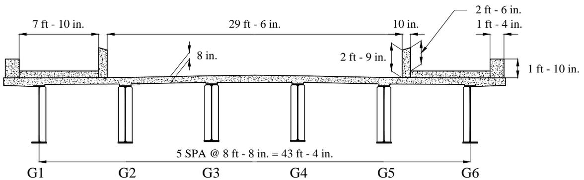
**Figure 3.3. Typical cross-sectional view of the E. 12th St. Bridge (looking north)**
