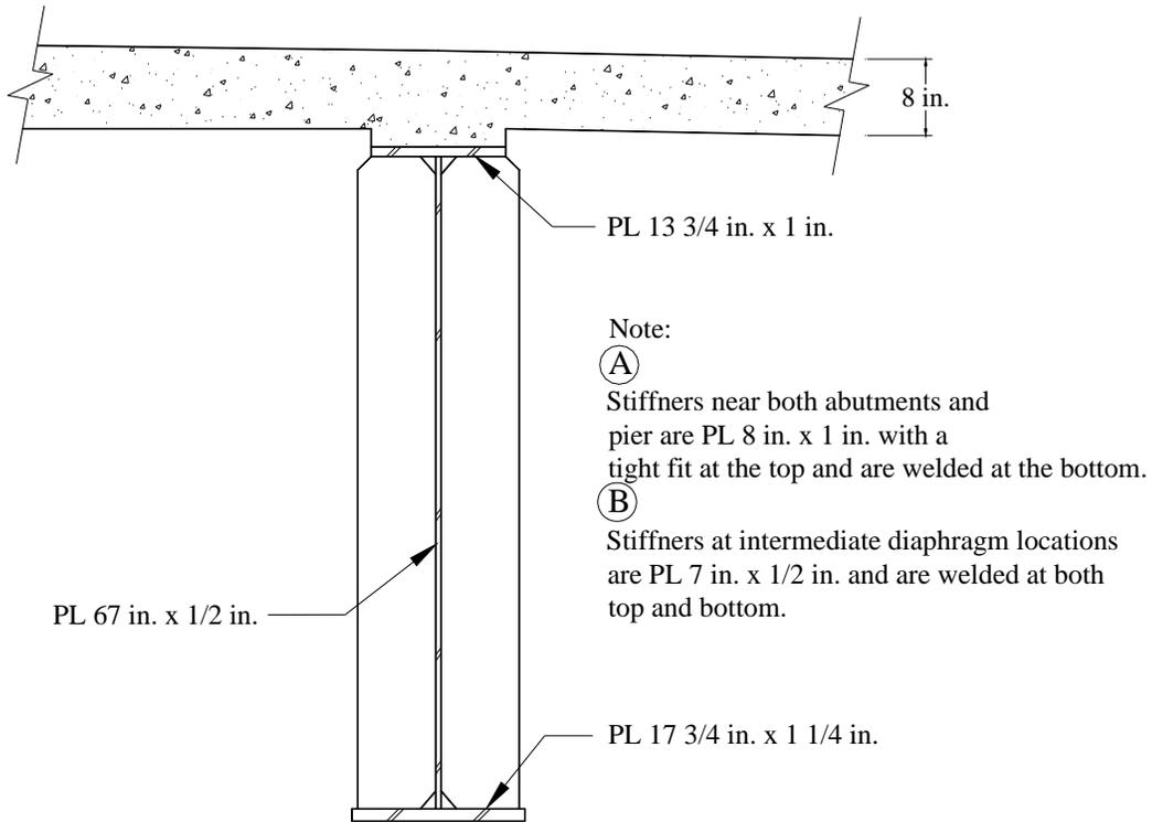
**Figure 3.4. Cross section of the “North Region” girders**
