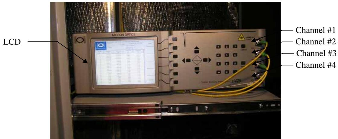
**Figure 4.16. Front panel of the Si425-500 interrogator**
