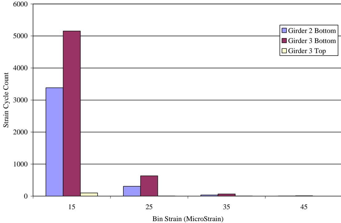
**Figure 5.39. Rainflow counting results from abutment sensors**
