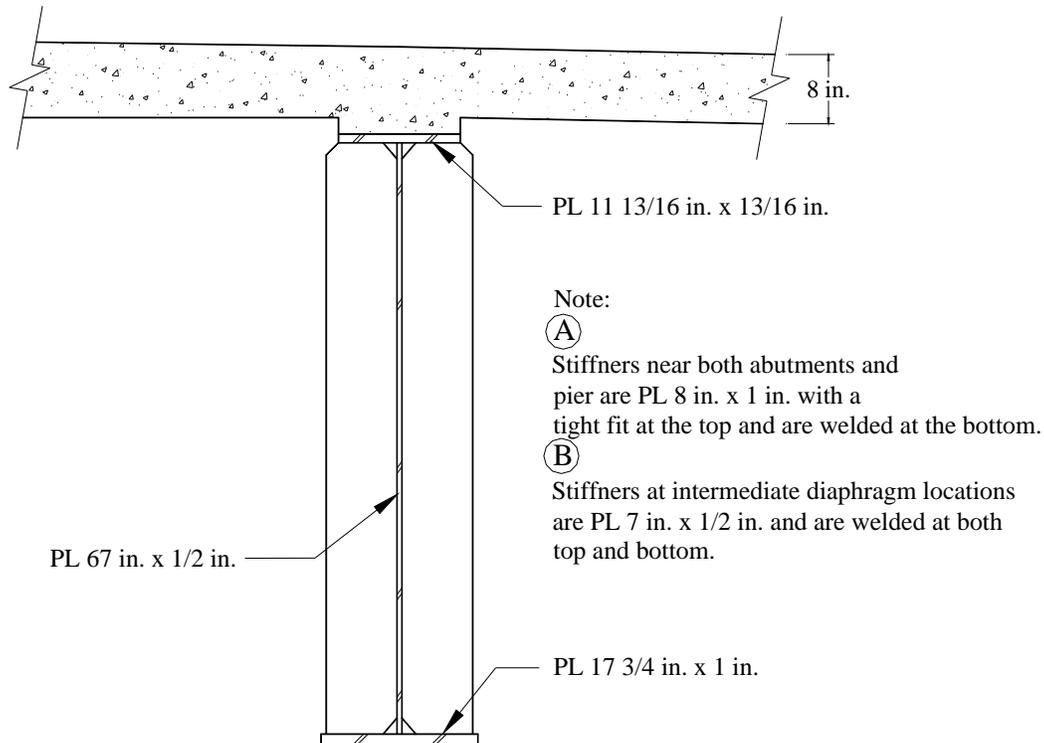
**Figure 3.6. Cross section of “South Region” girders**
