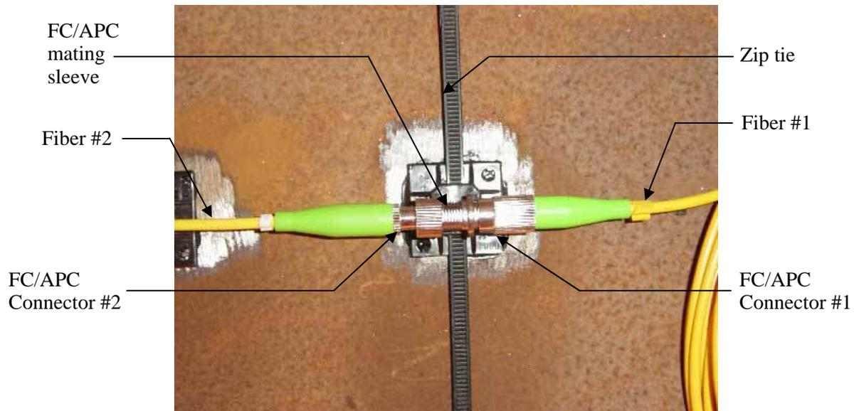
**Figure 4.12. FC/APC mating sleeve connecting two fibers**
