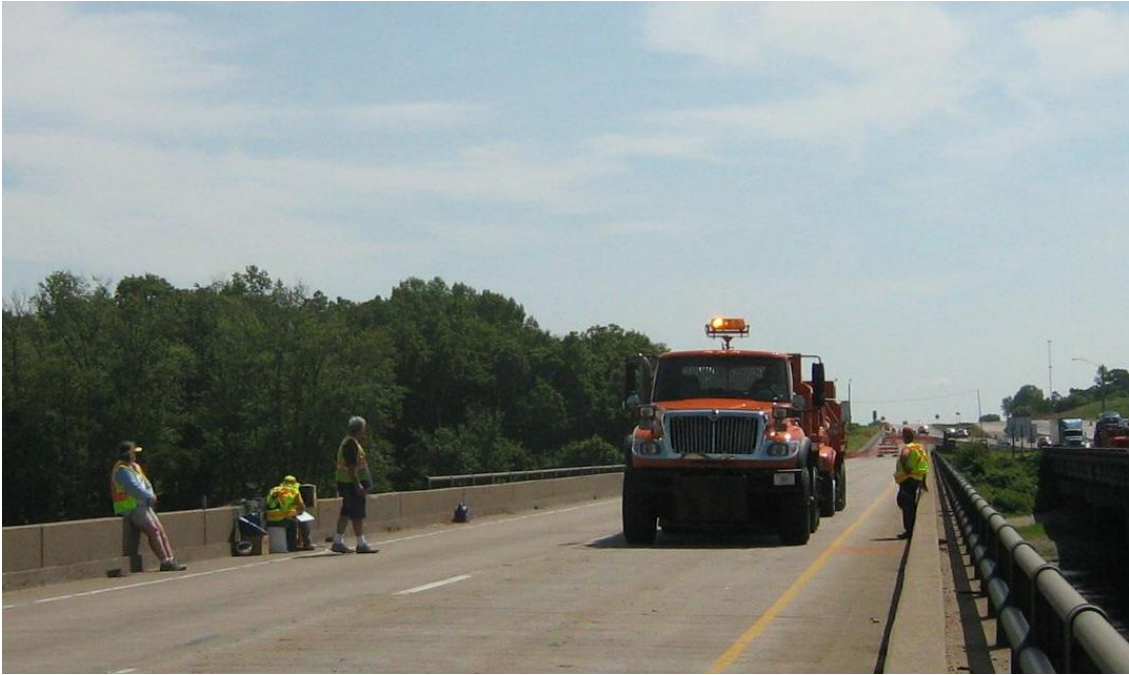
Figure 14. Load Case 7 (Truck 1 and Truck 2 back-to-back in middle lane). Trucks are separated by approximately 10 ft and are in the south lane.
