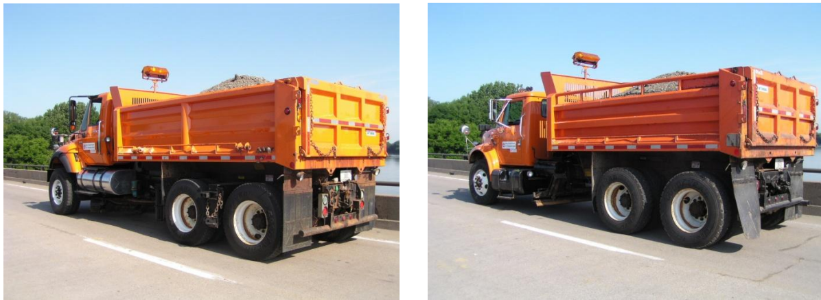
Figure 12. Load test dump trucks; Truck 1 and Truck 2, respectively. Truck 1 had weights of 16.6 kips for front axle and 38.4 kips for rear tandem axles. Truck 2 had weights of 13.2 kips for front axle and 34.0 kips for rear tandem axles.
