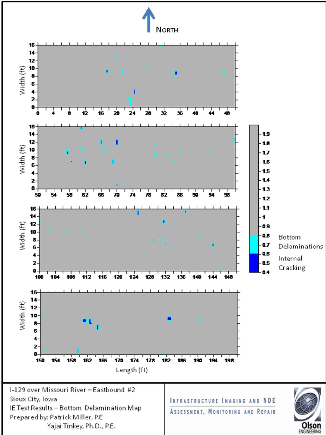
Figure C2 – Bottom Delamination Maps for Eastbound #2
