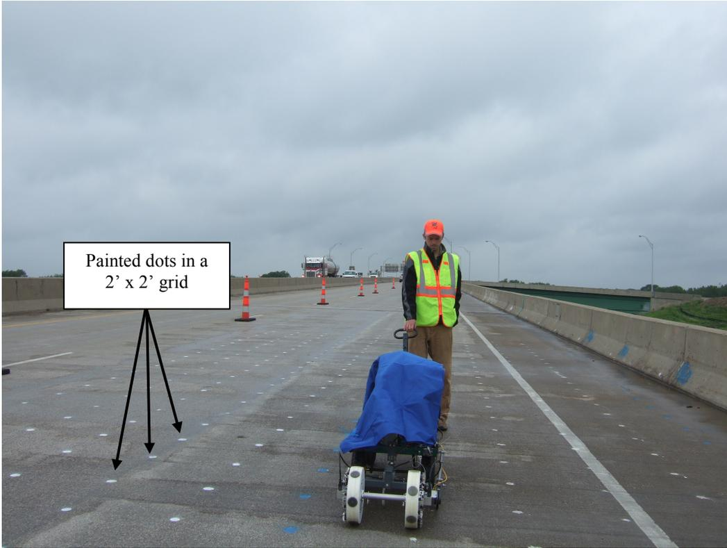
**Figure 2: Photograph showing test grid layout for BDS-IEtesting on a 1 ft grid with impacts every 6 inches to provide 1 test every 0.5 sq ft**
