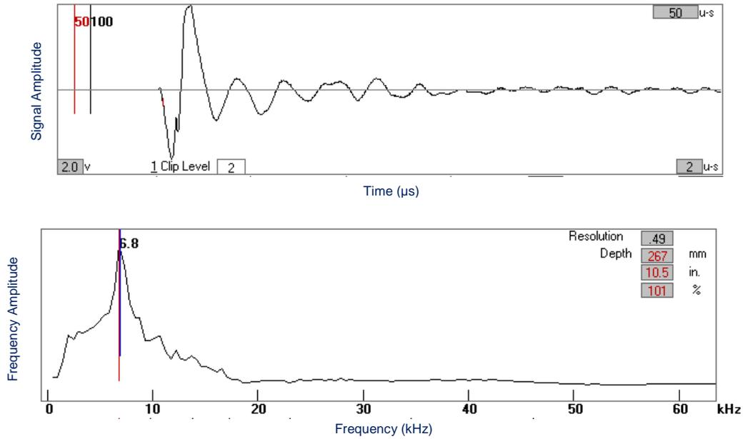
Figure 5.5. IE test result showing a reflection from the bottom of the deck at a depth of 10.5 in. (Study Area EB-1; Station 314).
