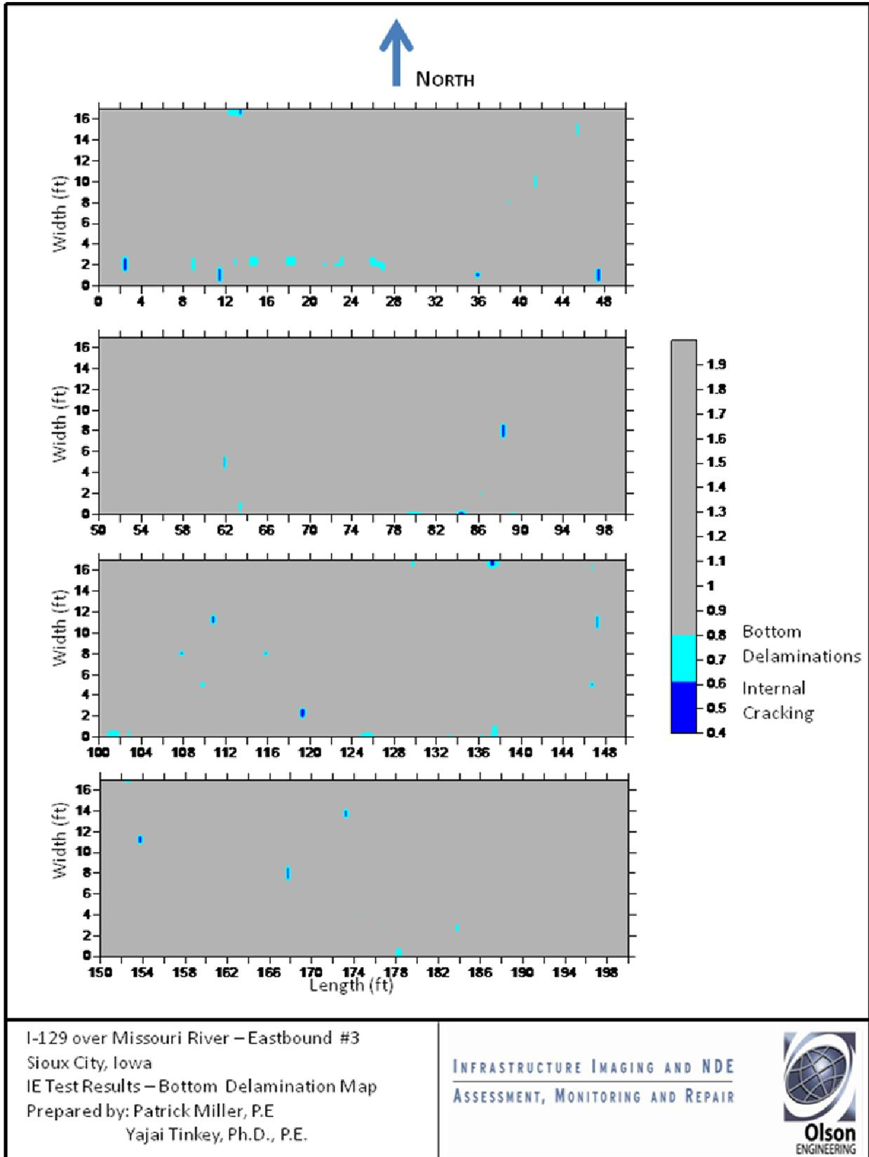
Figure C3 – Bottom Delamination Maps for Eastbound #3
