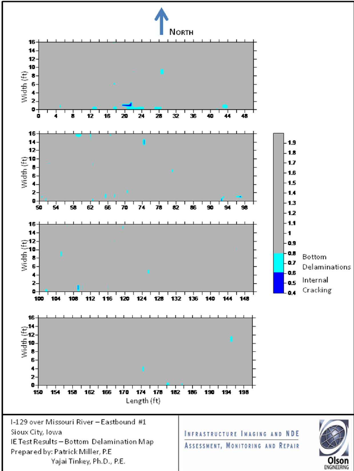
Figure C1 – Bottom Delamination Maps for Eastbound #1
