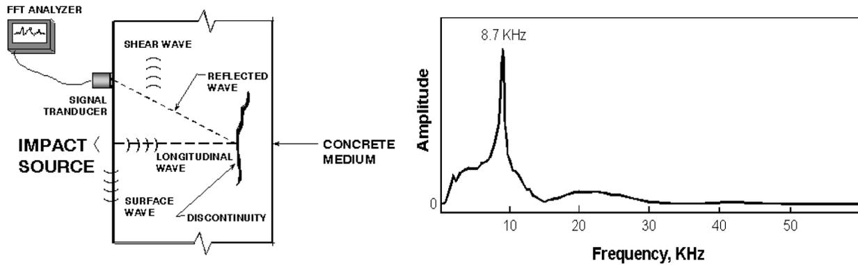
*Figure 5.1. Schematic of the Impact-Echo method. The general basis of the method is on the left, and a typical frequency spectrum plot is on the right. The dominant (resonant) frequency is then correlated with deck thickness or delamination depth.*
