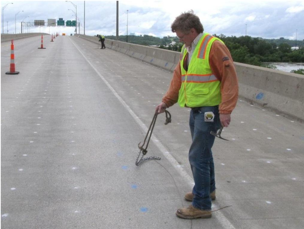
*Figure 2.2. Mechanical sounding.*
