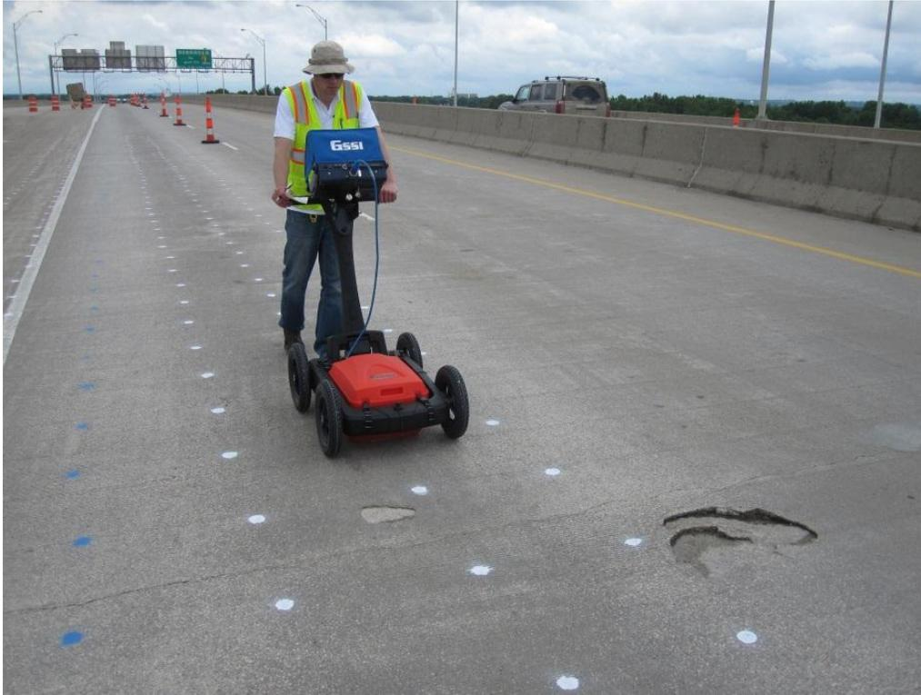
*Figure 4.1. GPR data collection within the WB-2 study area using the GSSI Bridgescan system.*
