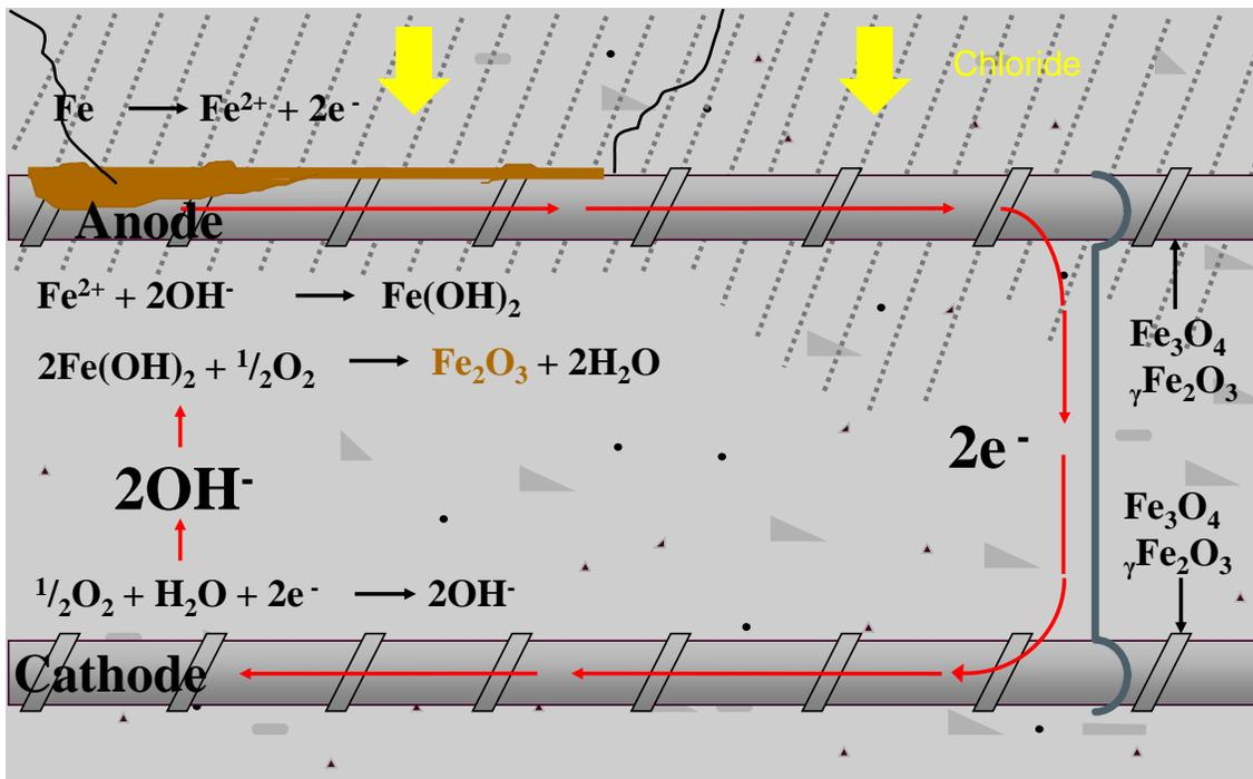
Figure 6.1. Sketch representing corrosion reaction in reinforced concrete.
