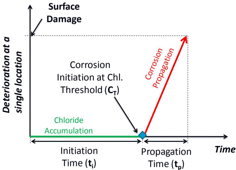
Figure 8.6. Corrosion sequence (adapted from Tuutti 1982).
