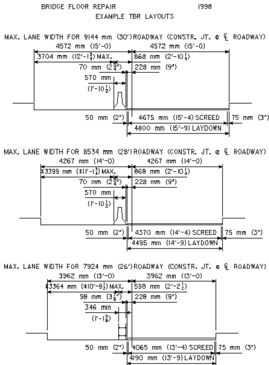
Figure note: All cases illustrated above require special signing because the roadway width is less than 14.50 feet between barriers. If the lane width is less than 10.50 feet the Traffic and Safety Bureau also will need to review the TBR design. See the manual text [BDM 12.1.8.3].
