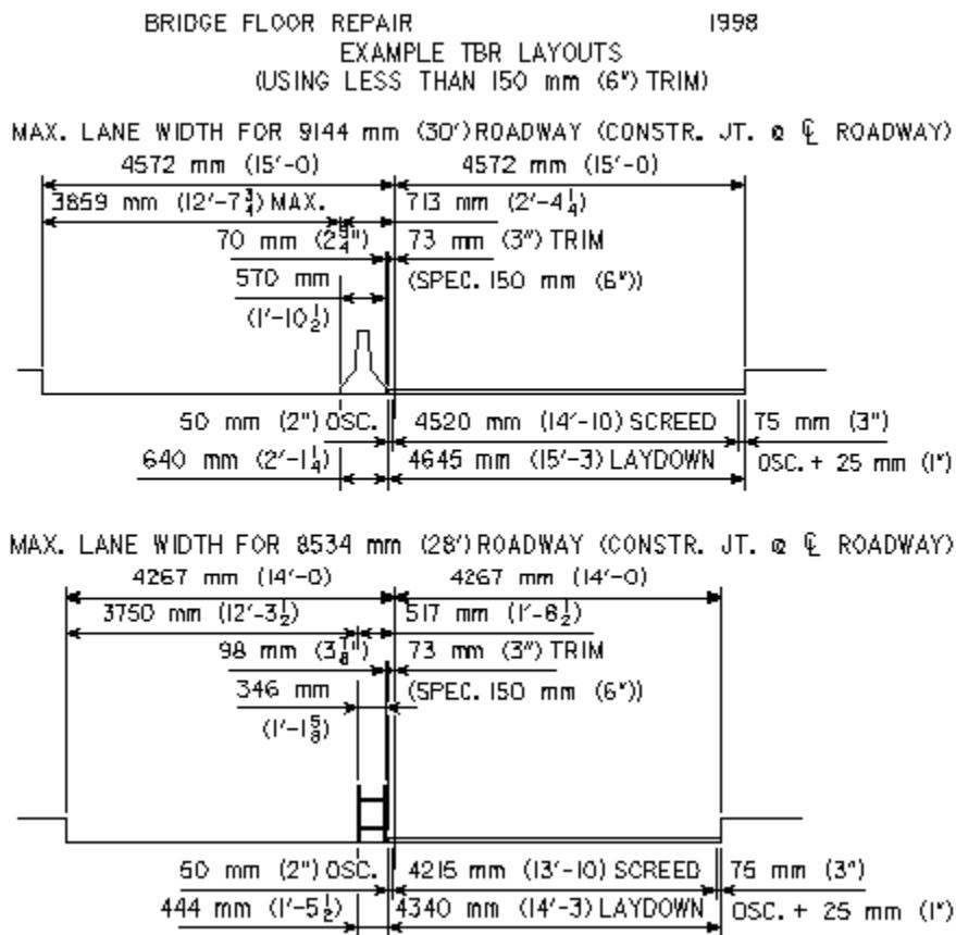
Figure notes: When less trim is used than required by the Standard Specifications, include deck repair note E432 [BDM 13.5.2]. Reduce trim only when needed to maximize roadway width.
